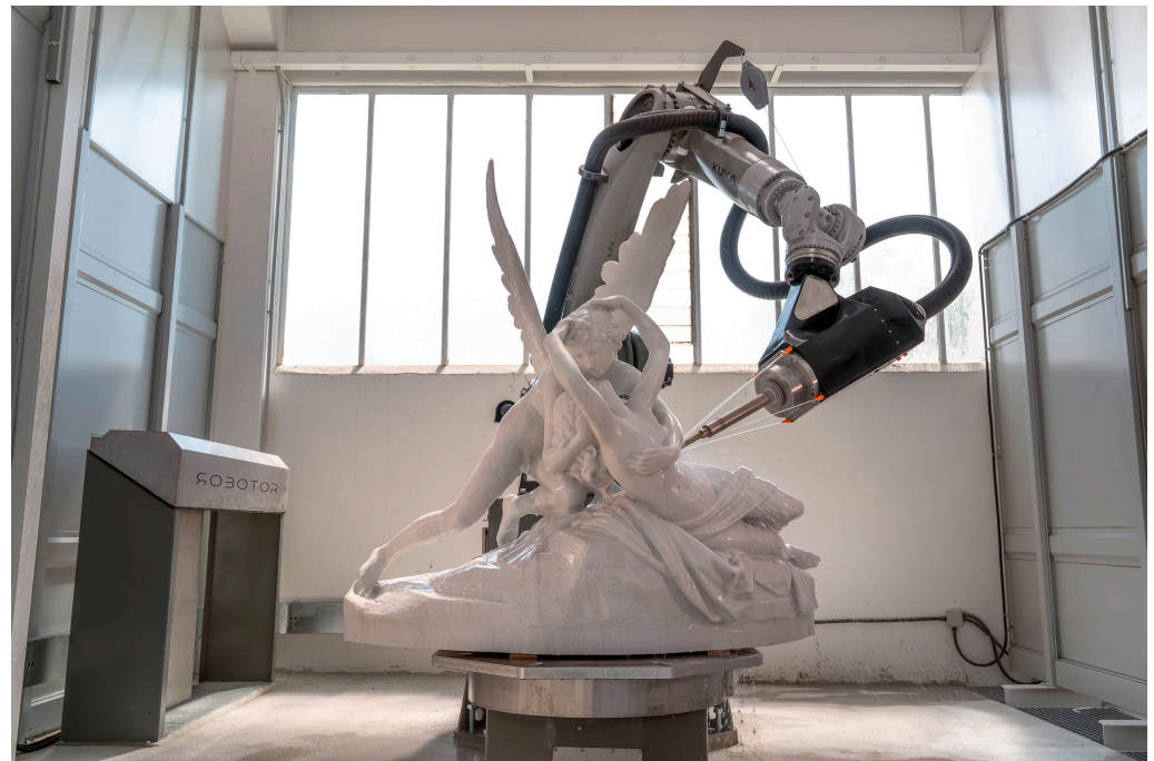
Figure 8. A reproduction of Canova’s Cupid and Psyche starting from a 10-ton block of white Carrara marble by the Robotor system. Reproduced with permission from [143].
