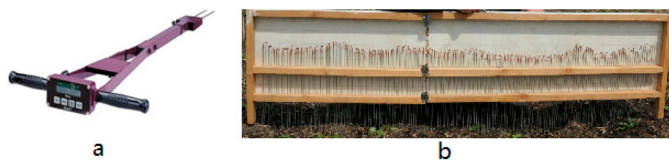
Figure 2. The procedure for measuring (a) soil moisture using TDR and (b) surface roughness profile.
