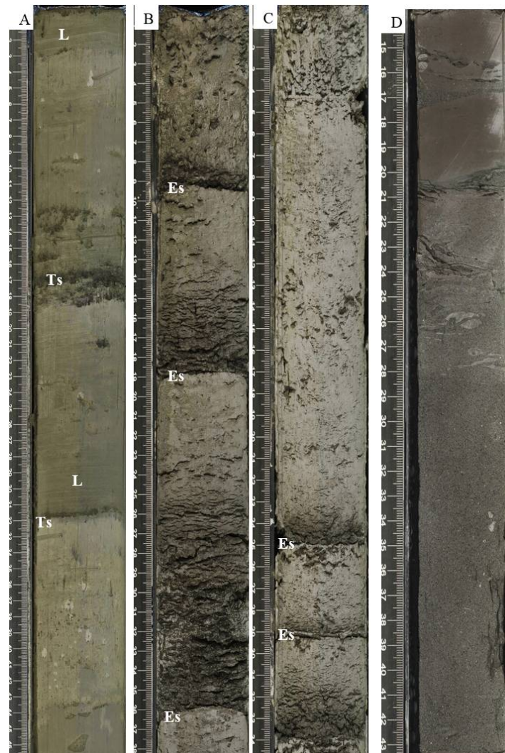
Figure 5. Core photographs of typical turbidite facies from site 1457 of expedition 355. The turbidite sequences are characterised by dark grey sandy silt or silt and normal grading to pale grey mud. Ts—thin layer of silty sand, Es—erosional surface, L—laminated. (A) 1457A-8H-2A; (B) 1457A-1F-1A; (C) 1457C-9R-1A; (D) 1457C-38R-2A.
