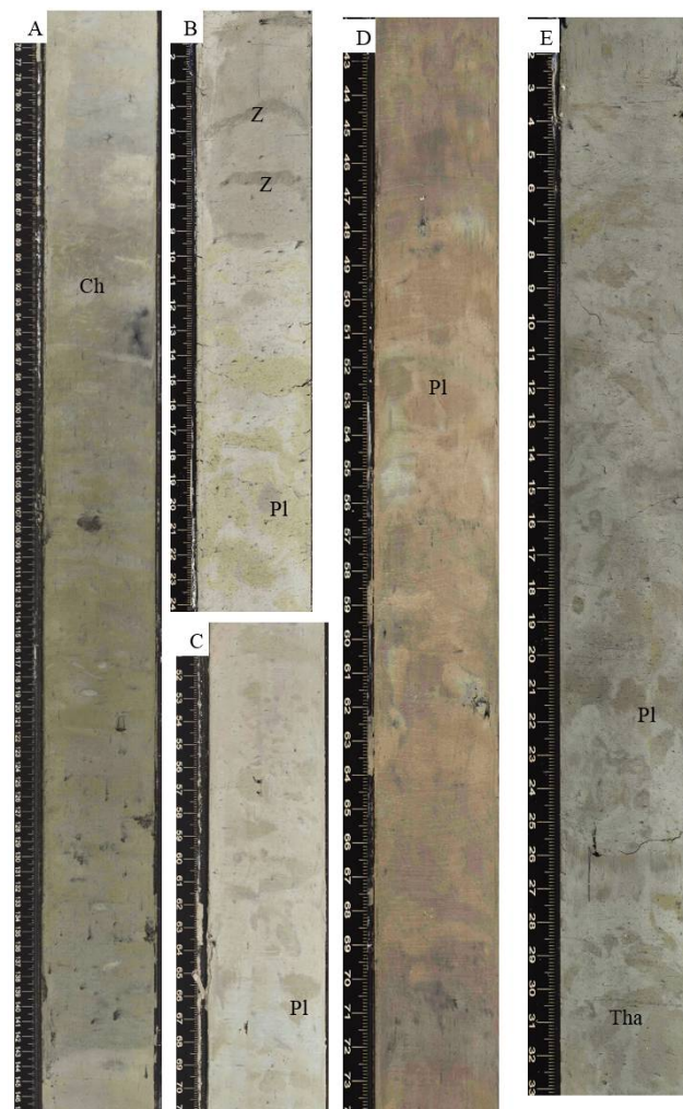
Figure 4. Core photographs showing typical hemipelagite facies from site 1385 of expedition 339 with pervasive mottling. The core photos display intense bioturbations and distinct colour cyclicity, in which lighter grey intervals have higher biogenic carbonate and darker grey intervals are rich in terrigenous components. Ch- Chondrites , Pl- Planolites , Tha- Thalassinoides , Z- Zoophycos . (A) 1385E-6H1-A; (B) 1385A-10H-7A; (C) 1385E-6H-1A; (D) 1385A-7H-1A; (E) 1385A-11H-3A.
