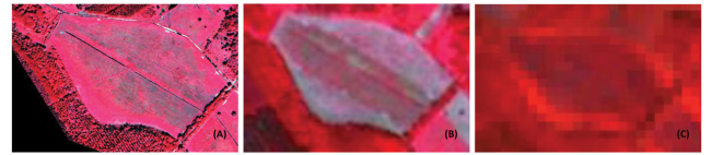
FIGURE 5. Spatial resolution comparison (false color composite: R = NIR, G = RED, B = GREEN) among QuickBird (A), RapidEye (B) and Landsat-8 (C) [75].
