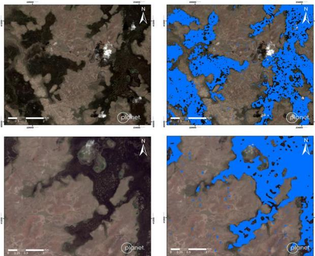
Figure 5. Example of the comparison of the SAR-CUSUM derived Open water detection mask (19<sup>th</sup> September 2020) with HR Planet image acquired on 20<sup>th</sup> September 2020.
