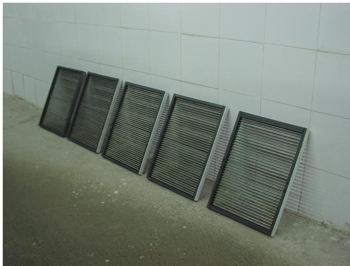
**Figure 5.1: Grading sheets designed for the experimental grading of gilthead seabream juveniles. The 5mm stainless steel bars are fitted into a plastic collar by holes drilled at fixed widths. The sheets are then slotted into a fibreglass box which holds the sheets 10cm under the water's surface. Gap sizes of the sheets were 1.5, 2.0, 2.5, 3.0 and 4.0mm; accurate to 0.1mm.**
