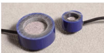
**Figure 3-3 BioPac Silver to Silver Chloride Electrodes**
