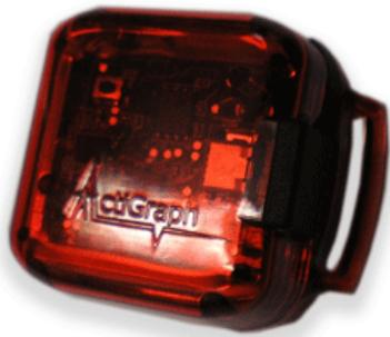
**Figure 3-4** GT1M Actigraph™ Accelerometer
