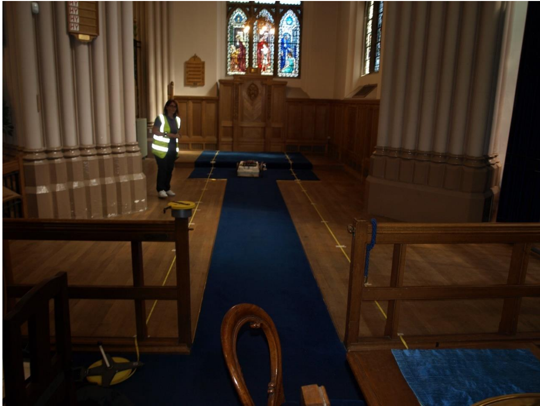
Figure 24: Survey Reference lines in the Memorial Chapel Reference line 1 to the left, line 2 to the right.
