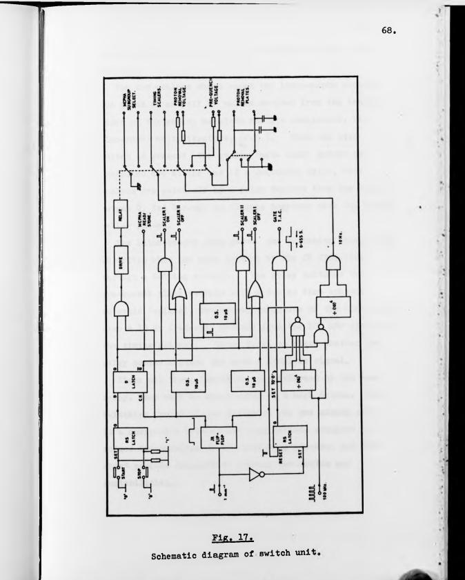
rest of the circuitry is then controlled by the latch outputs.
