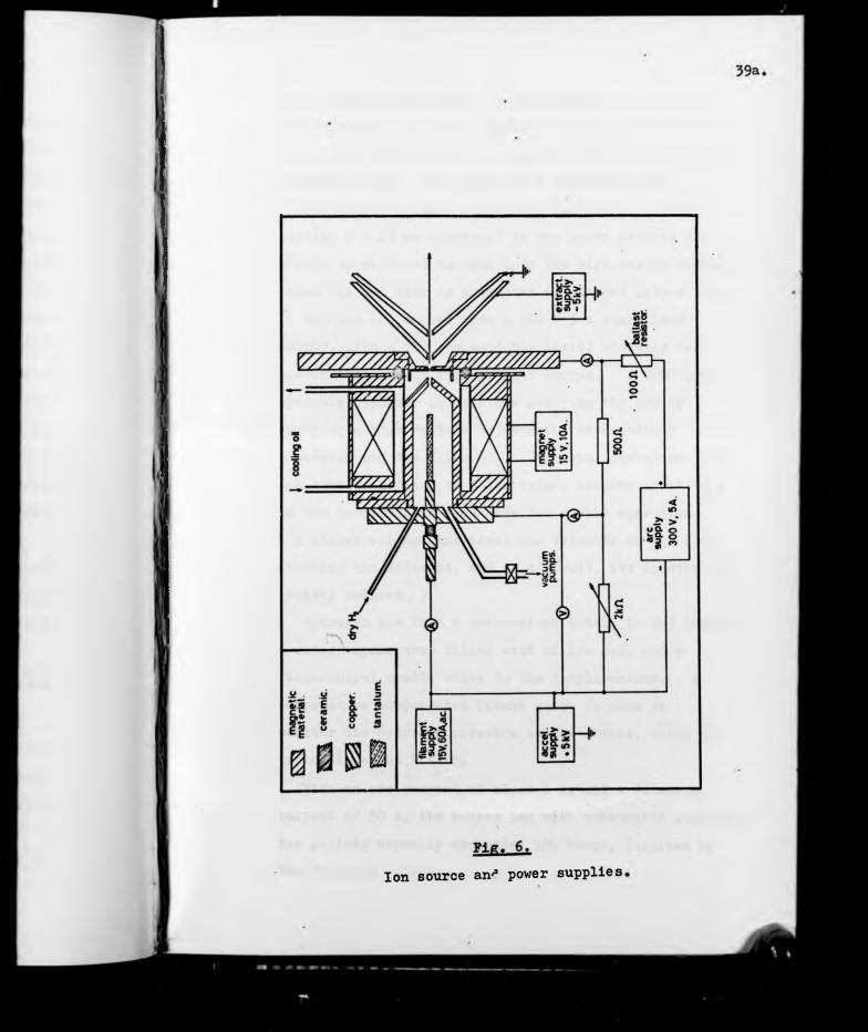
the filament and anode. An intermediate electrode constructed of magnetic stainless steel constricts the arc, which is focussed to a small area by a longitudinal magnetic field, thus producing a high degree of ionization in a small region at the anode. A small orifice ( 0.15 mm diameter) in the anode permits the plasma so produced to leak into the high vacuum region where the ion flux is extracted and shaped into a beam.
