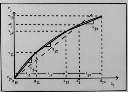
Figure 5.3. Piecewise linear approximation to the function V = f(G.) showing variables for a separable j programming matrix.
