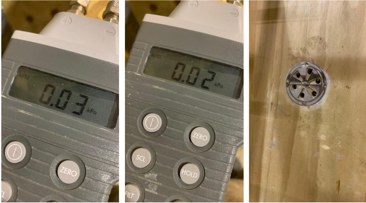
Figure 5.6. The boat vent (right) allowing pressure to be regulated to 20Pa, with a resolution of ~10Pa intervals.
