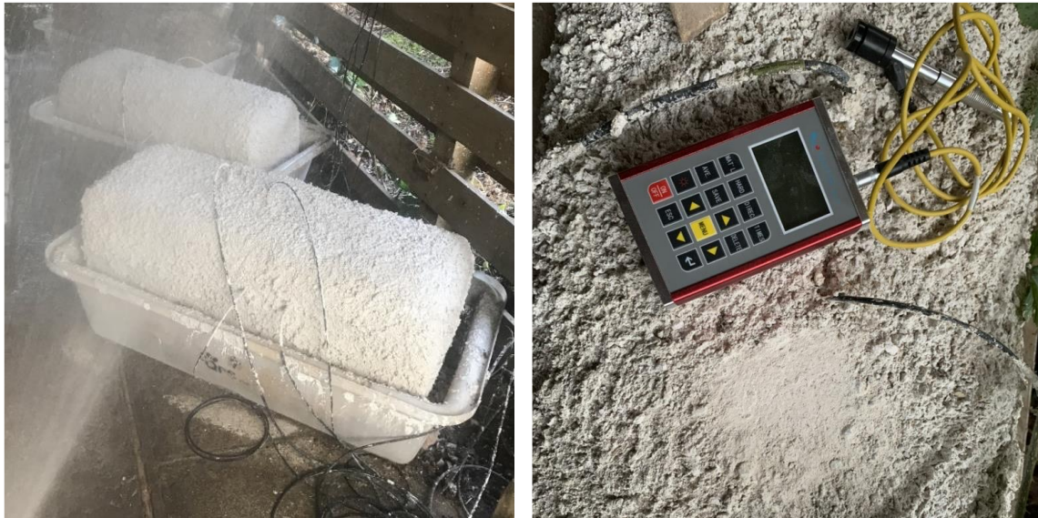
Figure 3.51. Earth blocks with Harl/Harl and limewash during LHT.
