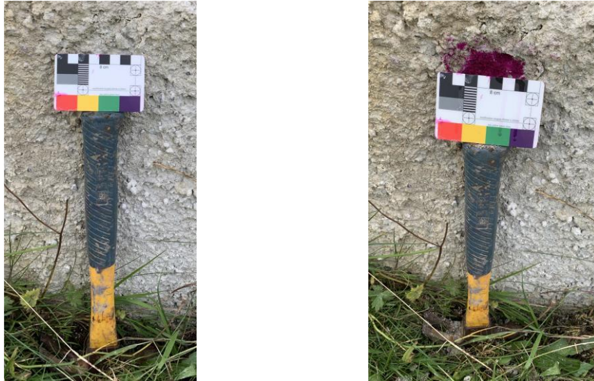
Figure 3.55. NE harled wall surface. Left: the carbonated surface sprayed with phenolphthalein. Right: with the outer crust teased away revealing the 2mm uncarbonated subsurface.
