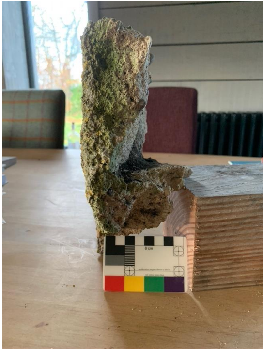
Figure 3.38. FT001. North elevation: harl with bedding tail.
