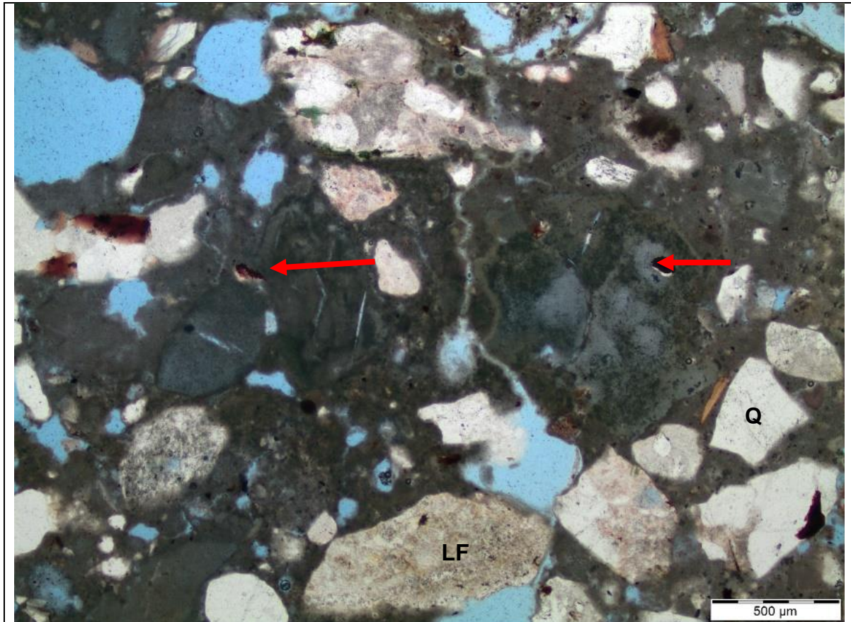
RB004A Two lime inclusions (red arrows) show partial dissemination into the surrounding mortar binder. The aggregate is comprised of lithic fragments (LF) and quartz grains (Q).
