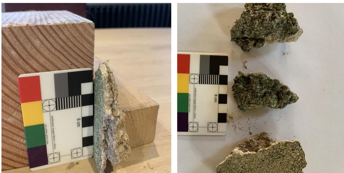
Figure 3.45. FT004ABC. Left: Detail of the line of separation between the 'polished' finished plaster and backing coat. Right: Core/bedding mortar, harled first coat plaster and 'polished' finish.
