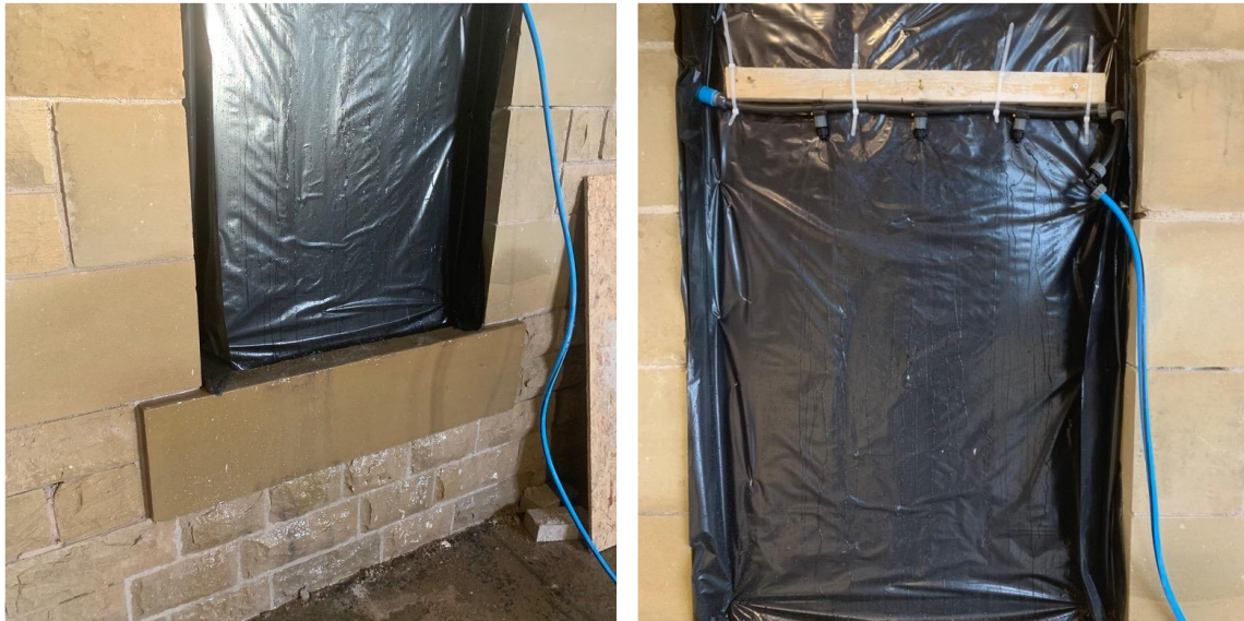
Figure 5.7. The 'window' frame showing the Visqueen membrane sealed to sides and base to simulate the windowpane. Right: Irrigation system.
