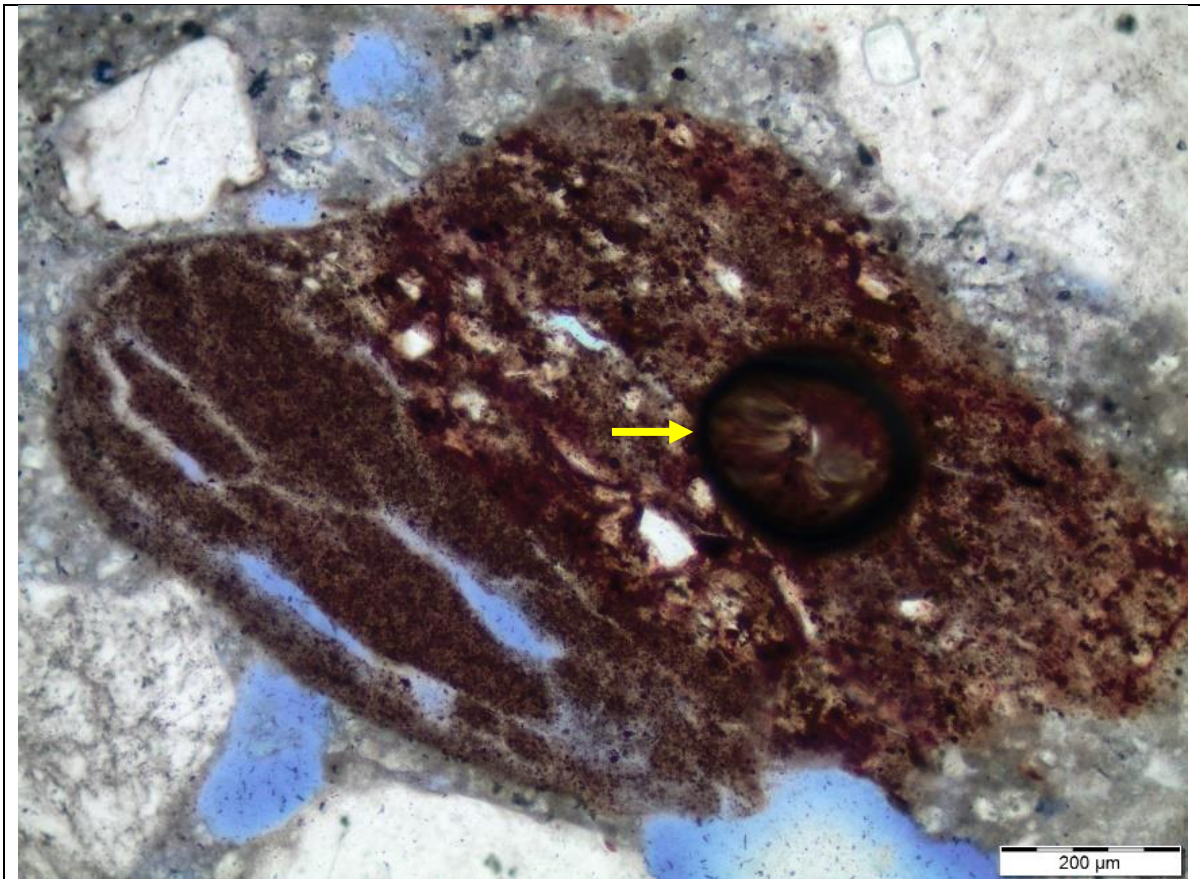
FT002 A small under-burnt lime inclusion displaying the relic marl limestone texture indicates the use of the same impure marl limestone in the manufacture of the mortar. The black circle (yellow arrow) is an artefact of the glass thin section slide. Note the scale bar shows 200 \mu m.
