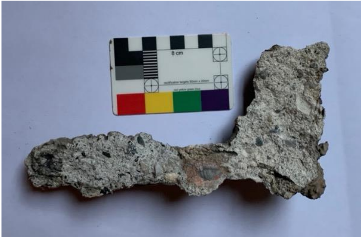
Figure 3.8. Bedding mortar (left) and harl (right) from the Lime Kiln at Port Ramsay, Lismore.
