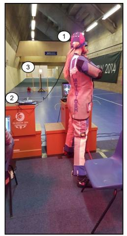
**Figure 4.1.** An example of the mobile real-world shooting experimental setup. [1] EEG sensors, [2] Amplifier, data storage unit and acoustic trigger box, [3] 10m Air-Rifle shooting target. Note that event triggers are implemented through an acoustic trigger box and through a manual button press from the experimenter.
