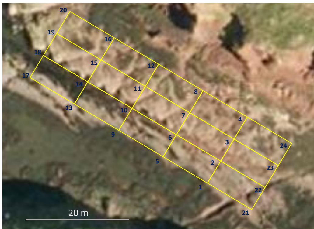
Figure 3.3. The gridded sampling sites of the “local scale” study. The distance lag is 5 x 10 m. Sampling sites are on the nodes of the grid.
