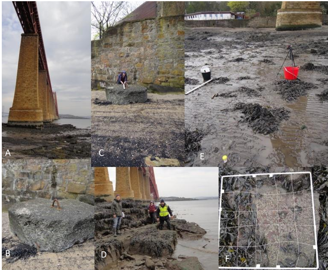
Figure 2.11. The South Queensferry sample locality. A: Sampling locality overview. B: The concrete cylinder used for site datum. C: Site datum and the reference for the furthest site. D: Part of the sampling team. E: A laser fixed to a tripod was used to measure the site. Yellow pots were used to mark each sample site. Barnacle covered rocks were collected in buckets. F: The 50 cm × 50 cm quadrat used for gathering information at each sampling site.
