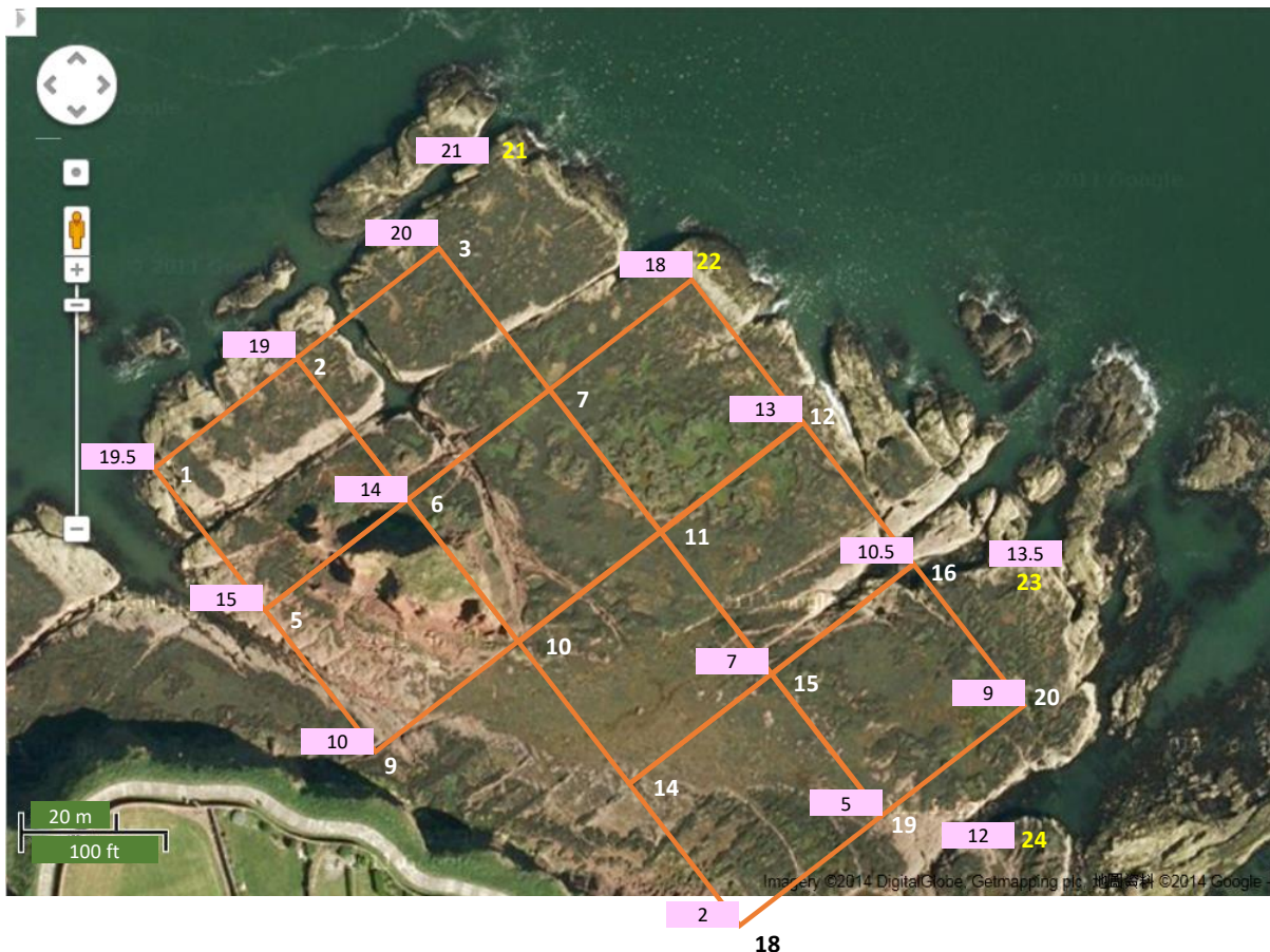
Figure 3.10. Ranking system in the whole area study. Each sampling point was given a rank by measuring the distance from site 18. Site 18 was designated as the reference site
