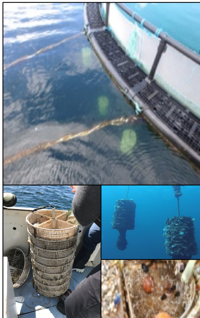
Figure 4-2 The photographs show the SBCC structures on the cage site. The photos below show the SBCC structures in water and off water. Photo on the right corner shows the fouling organisms inside an SBCC compartment.
