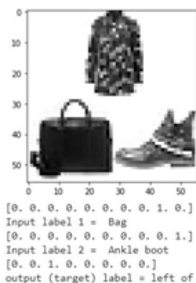
Figure 4: An example input and output encoding. In this example, the relationship "bag left of ankle boot" is represented.
