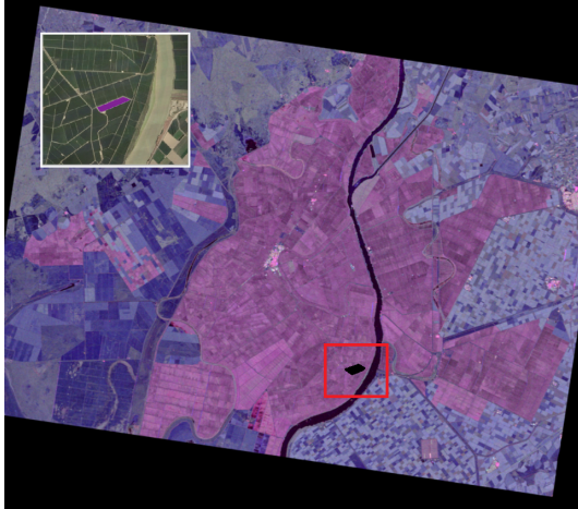
Fig. 1. Pauli RGB composite of the rice fields in Sevilla, Spain. RADARSAT-2 quad-pol data of 2014/08/16
