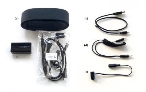
**Fig. 2.** The components of the MyndPlay BrainBandXL EEG Headset: (a) the headband on which the rest of the components are attached, (b) the unit that transmits via Bluetooth the EEG data to the computer, (c) the USB cable for charging the unit, (d) the two dry sensors attached to a soft material similar to the one used for the headband, and (e) the ear clip with the grounding electrode for the ear lobe.
