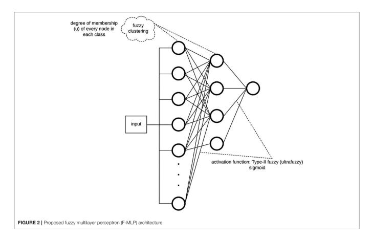
feature space. In fuzzy c-means (FCM), *X* is partitioned into *c* clusters by minimizing the objective function *J*:
