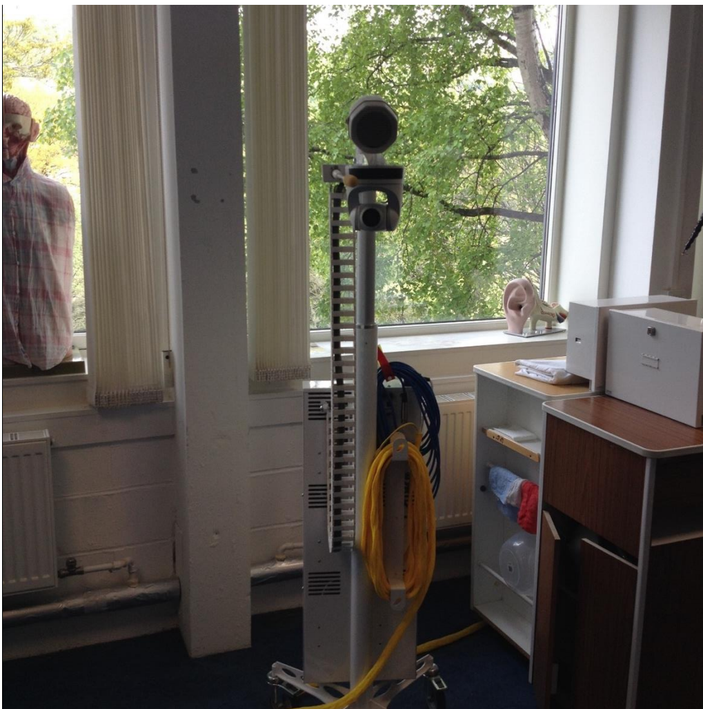
Figure 5: A mobile Smots™ camera housing a speaker and microphone linked via closed-circuit to the control room
