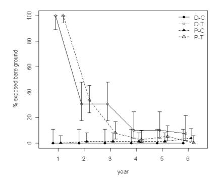
Figure 9.4 Change in exposed bare ground over six years at the two trial sites (Dorback (D) and Pentland Hills (P)) subject to initial scarification treatment, in control (C) and scarified (T) areas; 95% confidence intervals shown. Data points for the same year have been offset for ease of viewing.
