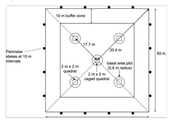
Figure 8.2 Plot layout used at both study sites (Inshriach and Novar) showing area thinned/clearfelled (for treatment plots) or left unthinned (for control plots), and locations of basal area (round) and vegetation (square) assessment quadrats.
