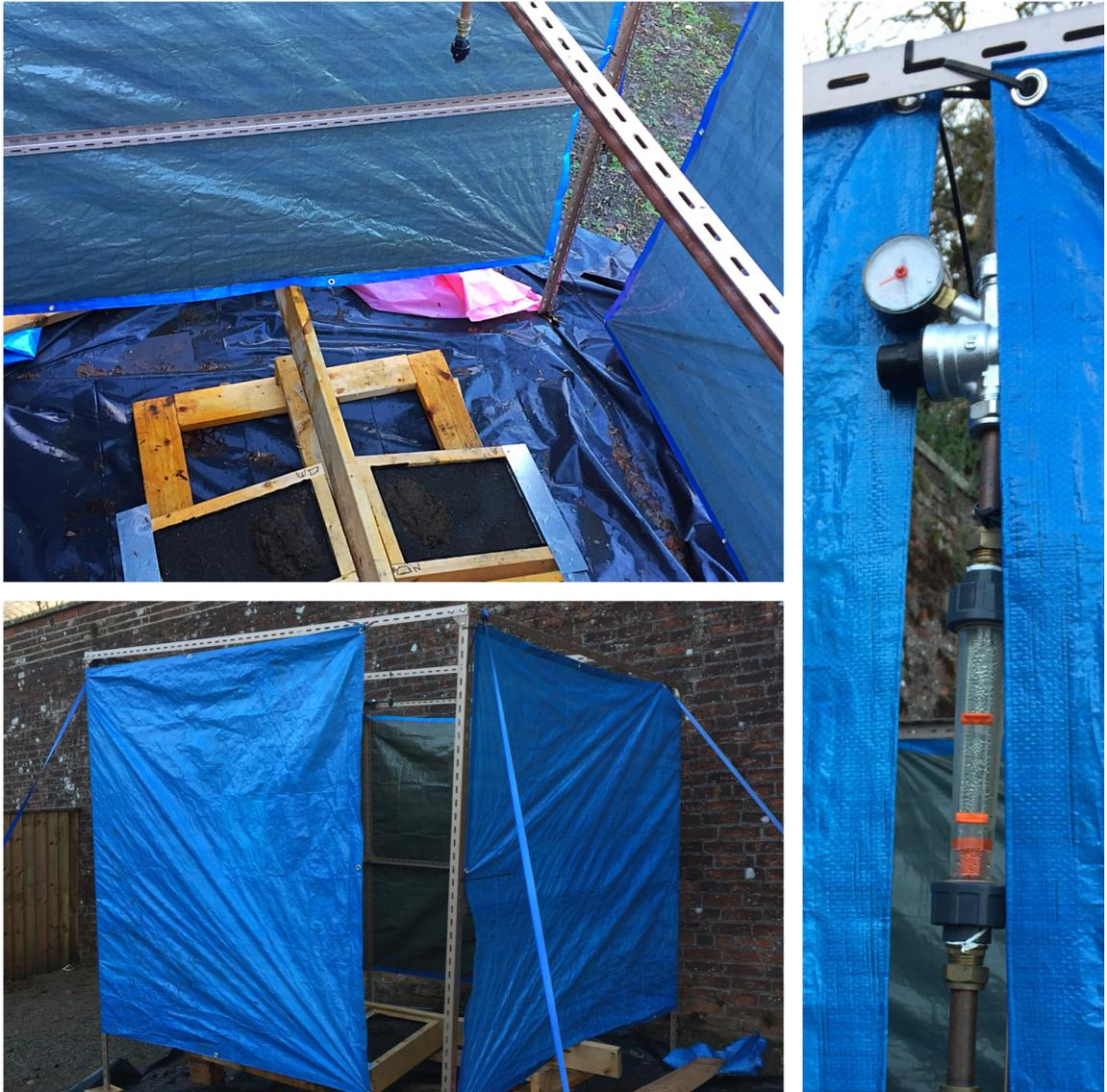
**Figure 5.1.** From the top left moving clockwise: placement of soil boxes underneath a spray nozzle; water pressure and flow gauges; rainfall simulator construction to prevent interference from wind.
