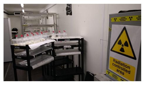
Figure 4.3 Radiation facility at Stirling University. Individual bumblebees in their housing were randomly assigned a radiation treatment. Different radiation dose rates generated by calculating distance from the <sup>137</sup>Cs source verified using an electronic personal dosimeter.
