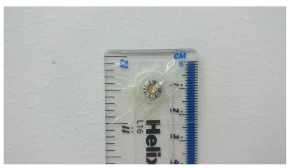
*Figure 3.4 Perspex ruler with inserted TLD to shield to allow contribution from beta and gamma radiation to be buried into the ground. TLD mounted at 10 and 30 cm.*
