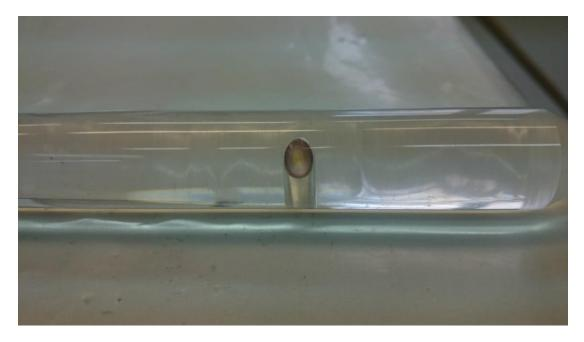
*Figure 3.3 One centimetre Perspex pole with inserted TLD to shield from beta and alpha radiation to be buried in the ground. TLD mounted at 10 and 30 cm.*
