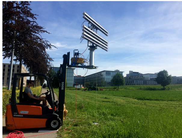
Figure 3. Hönggerberg experiment. The radar is mounted on a forklift to perform measurements at different elevations. In the near range, the lines of short cut grass separated by lines of piled grass and not yet mowed grass is visible. The observation area with a steeper slope is located at the far range and is not visible in the photograph.
