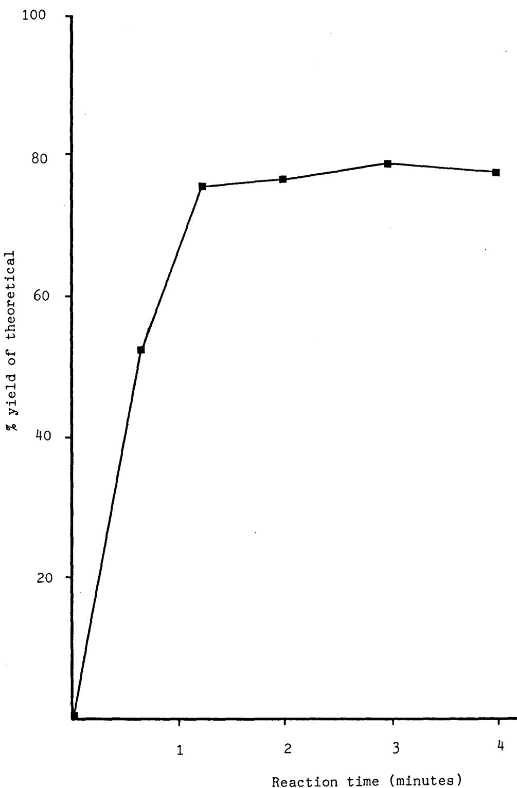
Fig. 2.7 Timecourse of ethylene release from 10 nmol authentic ACC in the presence of 200  $\mu$ l 15 mM  $HgCl_2$  and 400  $\mu$ l bleach/sat. NaOH. Final reaction volume in a 10 ml glass vial was 1 ml using distilled water to balance. Ethylene release was determined by headspace analysis.
