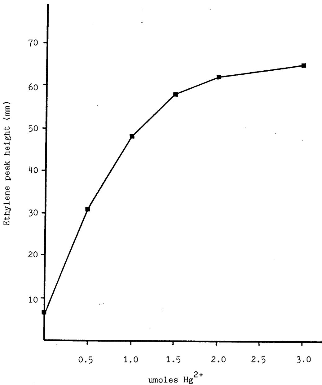
Fig. 2.10 Effect of  $\text{Hg}^{2+}$  on ethylene release from 400 ul ripe drupelet extract in a reaction mixture also containing 400 ul bleach/sat. $\text{NaOH}$ . The final reaction volume was maintained at 1 ml with distilled water. Reaction time 3 minutes in a 10 ml glass vial prior to headspace analysis for ethylene.
