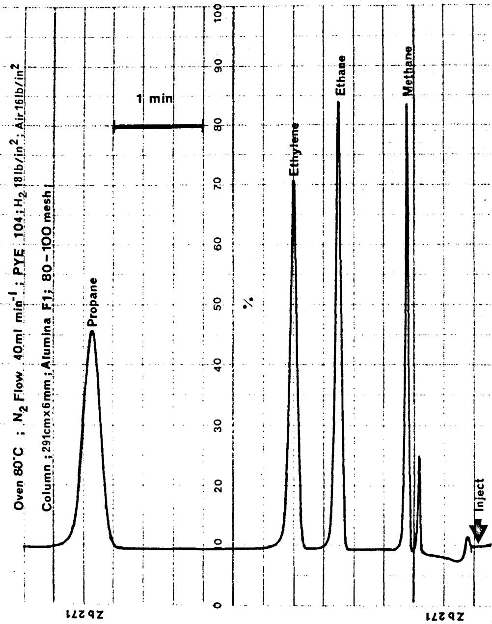
Fig. 2.2 Sample trace of optimum hydrocarbon separation using the Pye 104 Gas Chromatograph. Ethylene peak from 1 ml of 5 ppm ( $\mu\text{l l}^{-1}$ ) ethylene, the other peaks are from a hydrocarbon mixture, each of approximately 0.1%.
