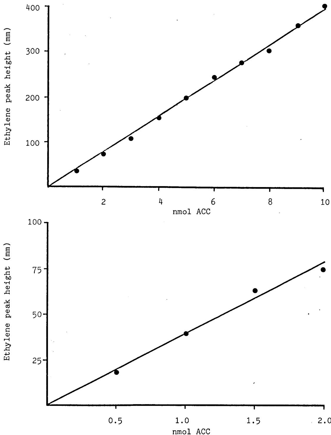
Fig. 2.6 Ethylene release from authentic ACC. Reactions carried out in 10 ml glass vials, final reaction volume of 1 ml containing 400  $\mu$ l NaOCl/sat. NaOH and 200  $\mu$ l of 15 mM  $HgCl_2$ . Headspace (1 ml) analyses for ethylene by G.C. after 3 minutes reaction.
