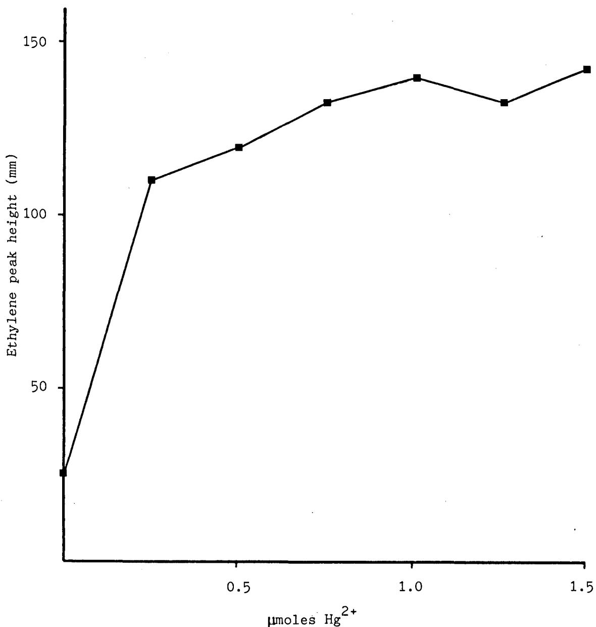
Fig. 2.9 Effect of  $\text{Hg}^{2+}$  on ethylene release from 2 nmol authentic ACC in a reaction mixture also containing 400  $\mu\text{l}$  bleach/sat. $\text{NaOH}$  in a final reaction volume of 1 ml, the balance being distilled in water. Reaction time was 3 minutes in a 10 ml glass vial prior to headspace analysis for ethylene.
