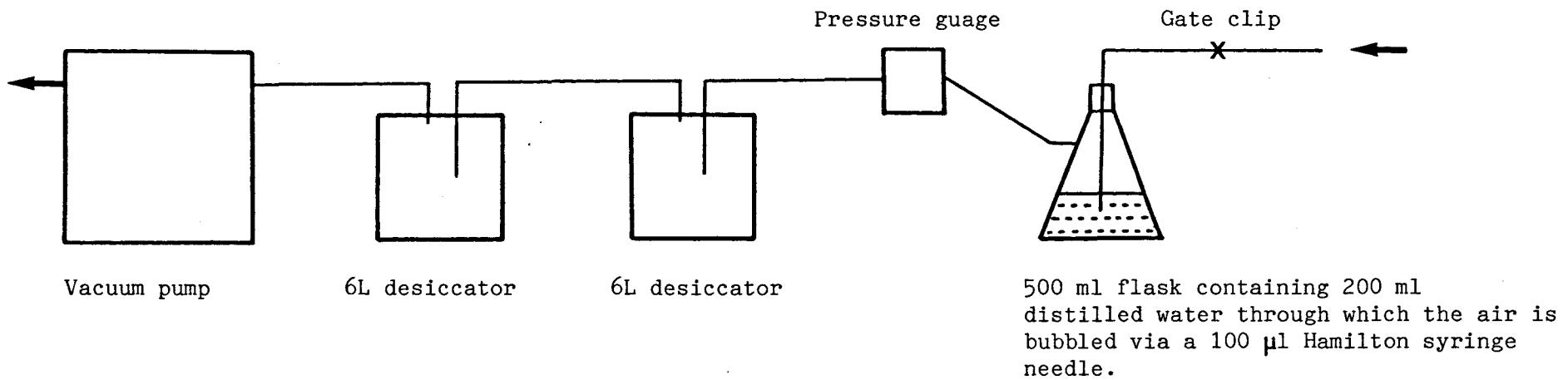
Fig. 2.5 Diagrammatic representation of the apparatus used in hypobaric treatments. Reinforced tubing was used to link the conical flask pressure guage and desiccators to the vacuum pump.
