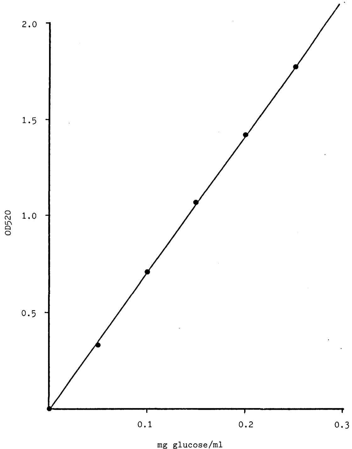
Fig. 2.4 Calibration curve for the OD520 resulting from the reaction of known amounts of glucose in the Nelson-Somogyi reducing sugar assay.
