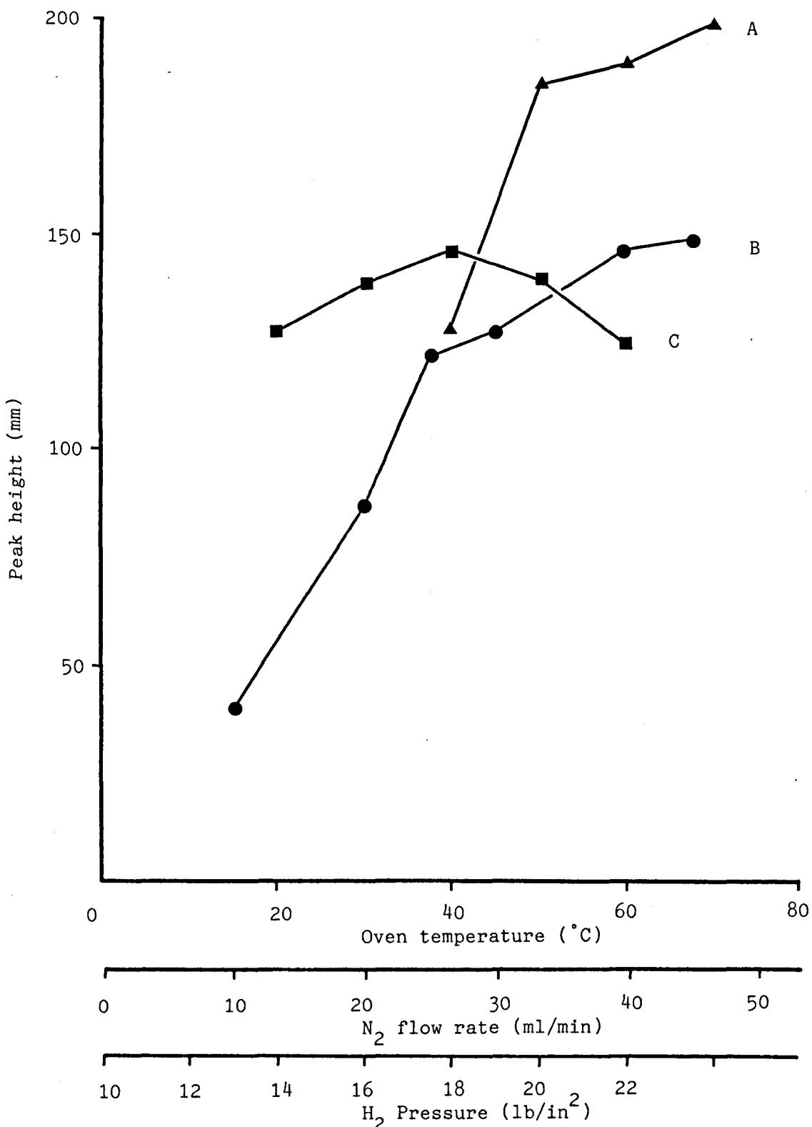
Fig. 2.1 Effect of changing different machine variables in maximising peak height of 1 ml of 5 ppm ethylene injected onto a 200 cm x 3.5 mm Alumina F<sub>1</sub> column attached to a Perkin Elmer F11 G.C.
