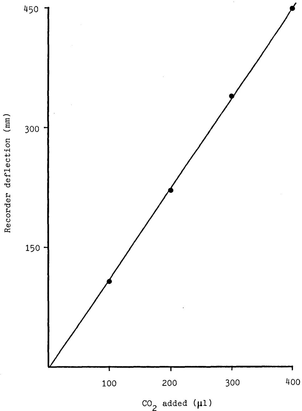
Fig. 2.3 Effect of cumulative additions of  $100 \mu\text{l}$  of carbon dioxide to a sealed atmosphere monitored for carbon dioxide by IRGA.
