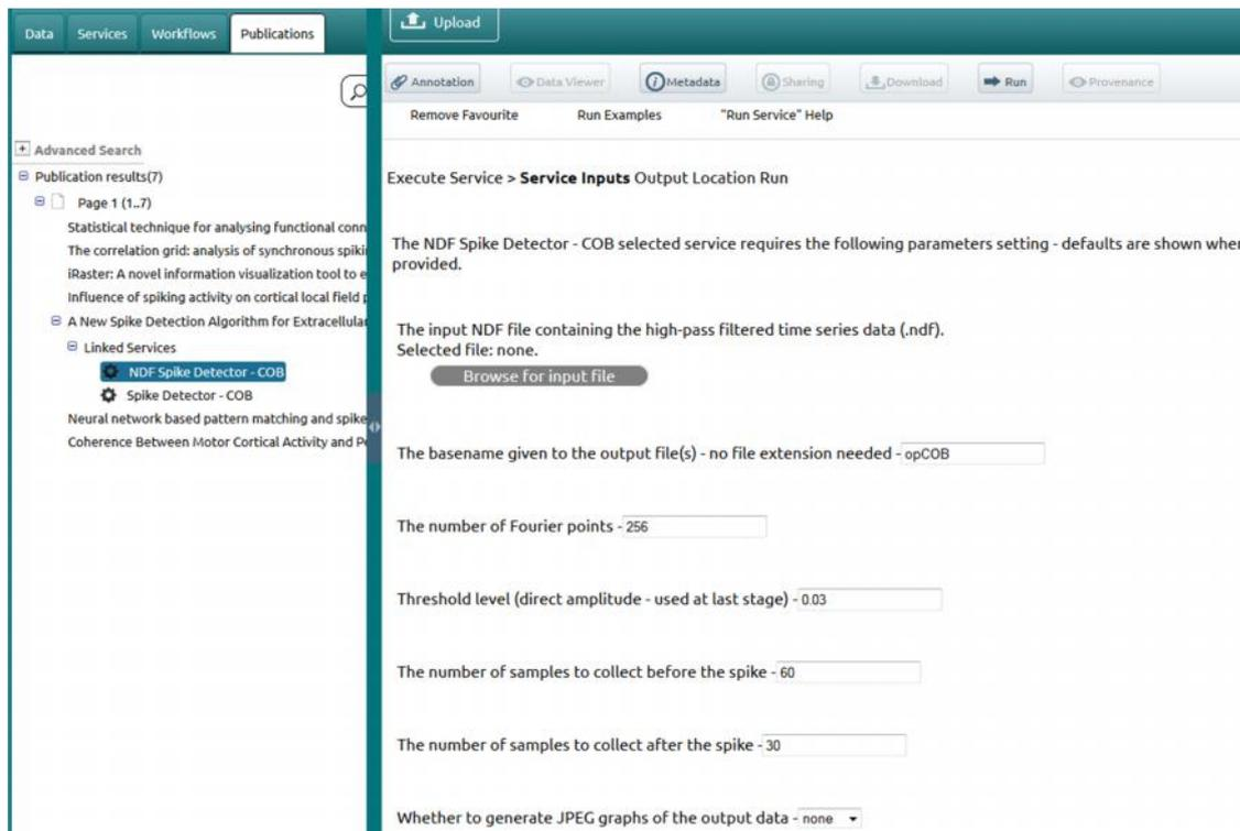
**Figure 9** The CARMEN VL provides reproducible results. The service can be prepopulated with data files and settings. In this screenshot, the parameter values are set but no input file is specified. However, the service requires an NDF type input file so the user will only be able to select a file of this type to ensure correct operation of the service. When the user selects the service, they can then execute the service as it was executed for the publication.
