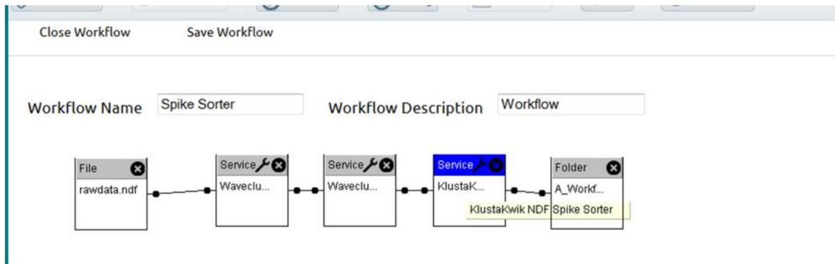
**Figure 2** Screenshot of an example workflow for spike detection. The data feeds into a Wave\_clus high pass filter, followed by a Wave\_clus spike detector (Quiroga et al., 2004), the spikes are sorted using a Klustakwik spike sorter (Harris et al., 2000) and the results are output to a selected folder.
