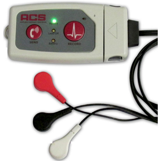
Figure 2 Example of a three-lead ambulatory ECG Holter monitor fitted privately by participants and worn from start of pre-assessment session to end of post-assessment interview
