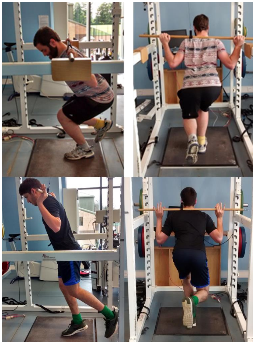
Figure 3.3 Unilateral CMJ. The wooden beam was used to control the depth of the squat phase, and was attached to a linear transducer to record displacement. CMJs were performed on a force platform.
