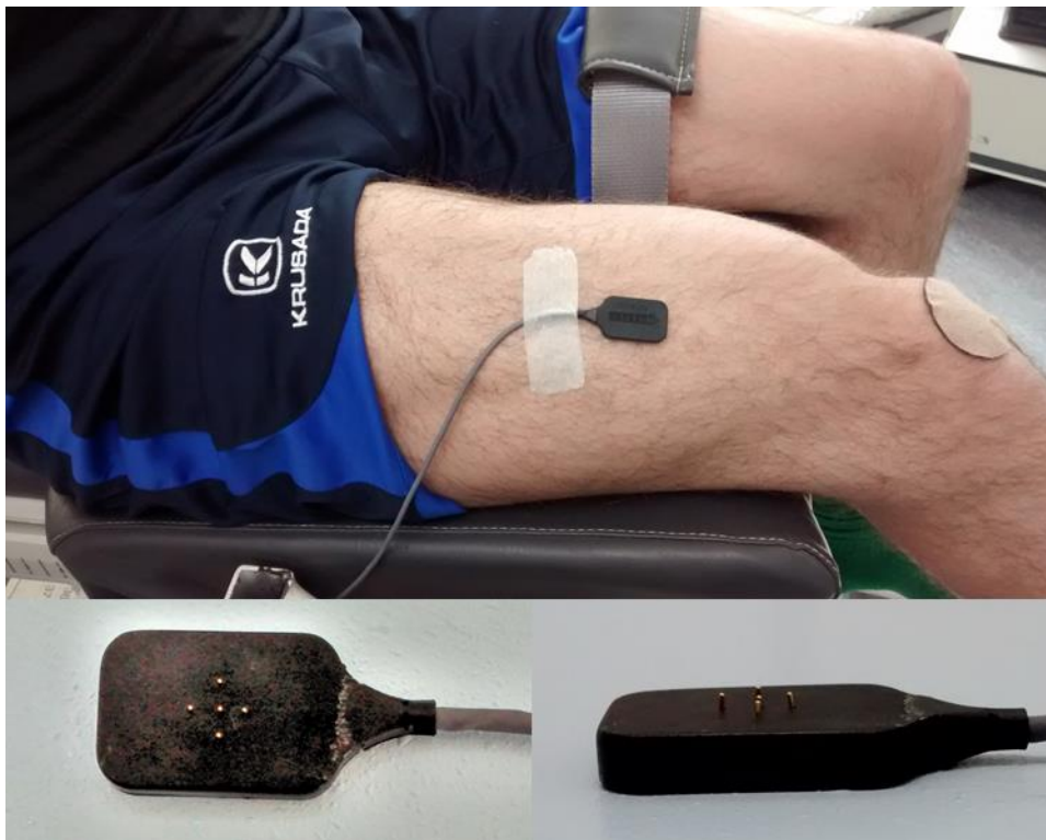
Figure 4.1 The surface array dEMG sensor (Delsys, Inc., Boston, Massachusetts) used to detect bipolar sEMG signals, on four separate channels. The sensor consists of five cylindrical pin electrodes, each 0.5mm in diameter, protruding from the housing (2x3cm).
