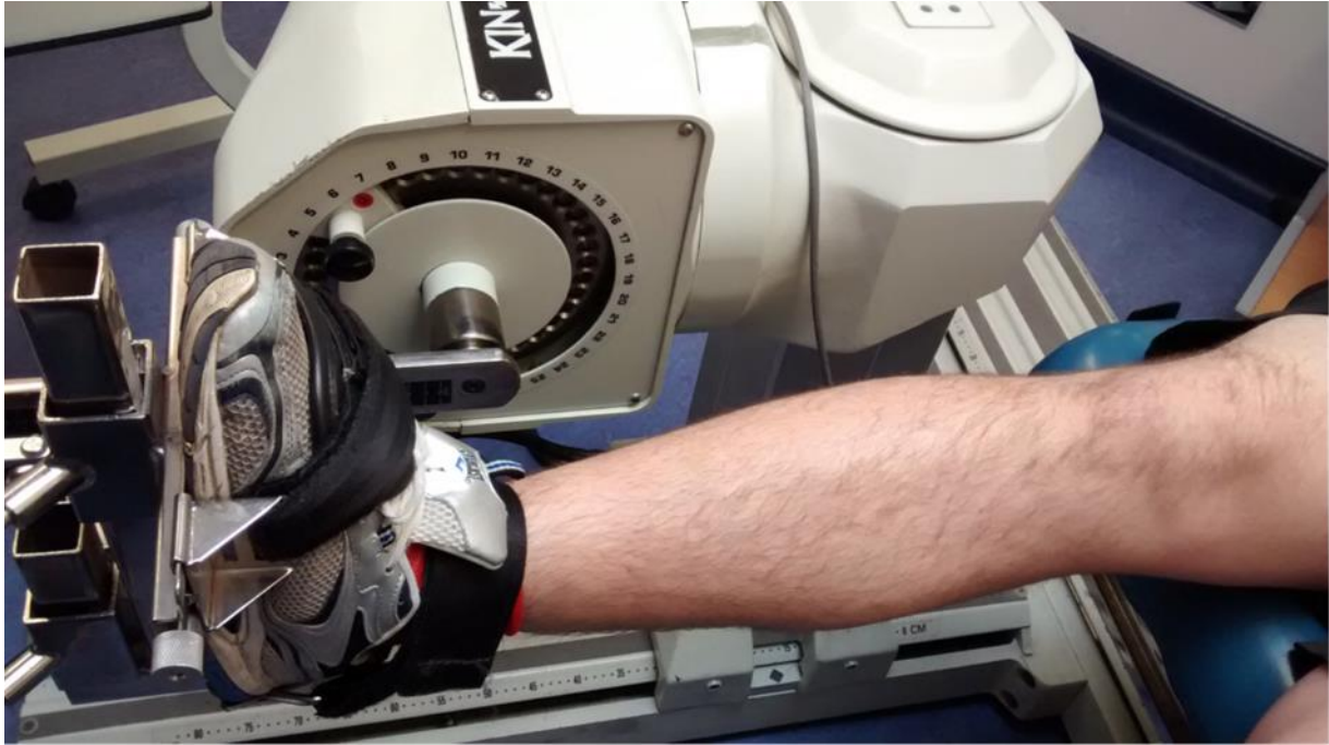
Figure 2.3 Isokinetic dynamometer setup for RMT and MVC assessment. Ankle flexed at 90° relative to the tibia
