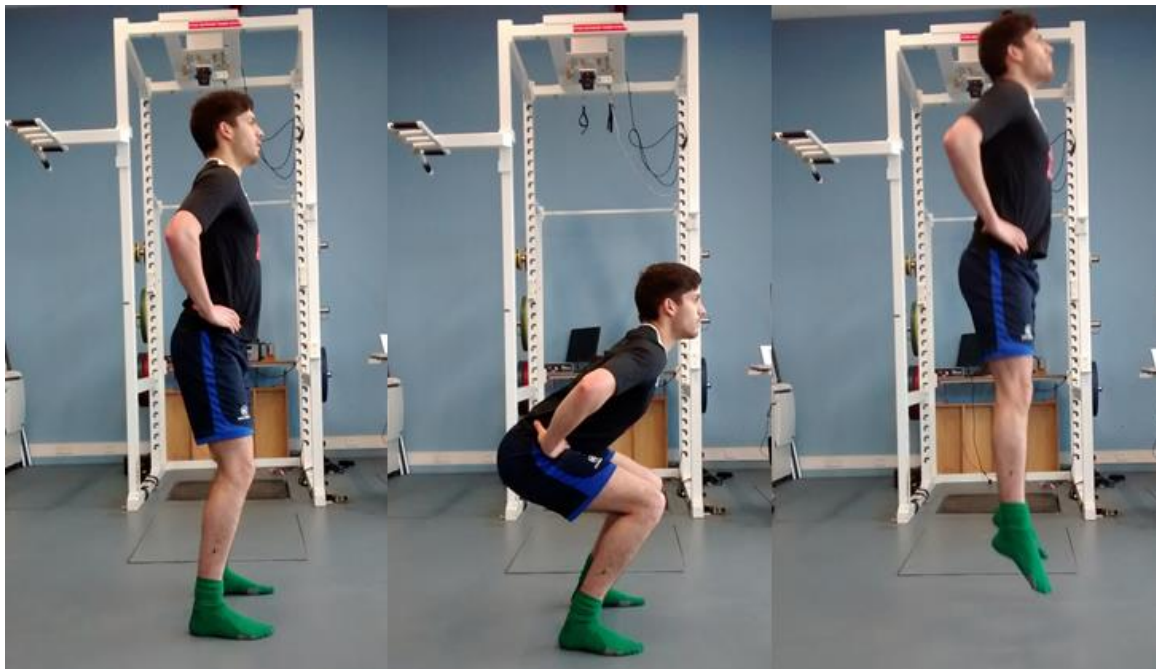
Figure 1.8 Vertical jump test, performed as a countermovement jump (CMJ).
