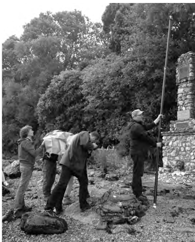
FIGURE 2: LEFT – THE GROUP CAPTURING IMAGES FOR PHOTOGRAMMETRIC MODELLING. RIGHT – A SCREENSHOT OF THE COMPLETED MODEL.
