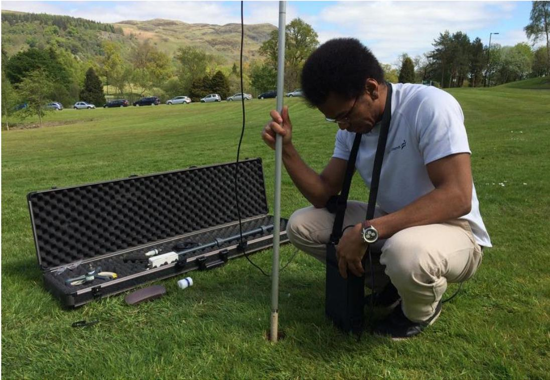
Fig. 3.15. Field operation of the Bartington MS2 magnetic susceptibility meter with the MS2H downhole sensor
