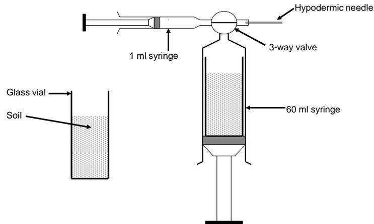
Fig. 3.17. Respiration chamber set-up for substrate-induced respiration experiment
