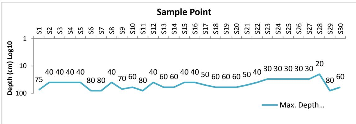
Fig. 7.21. Maximum profile depth of individual sample points across the site
