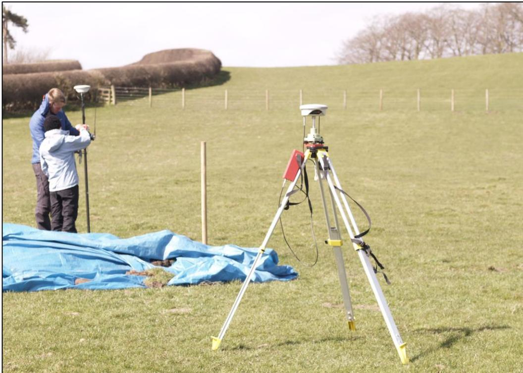
Fig. 3.18. Leica GS09 differential GPS unit being utilised in the field at Roxburgh
