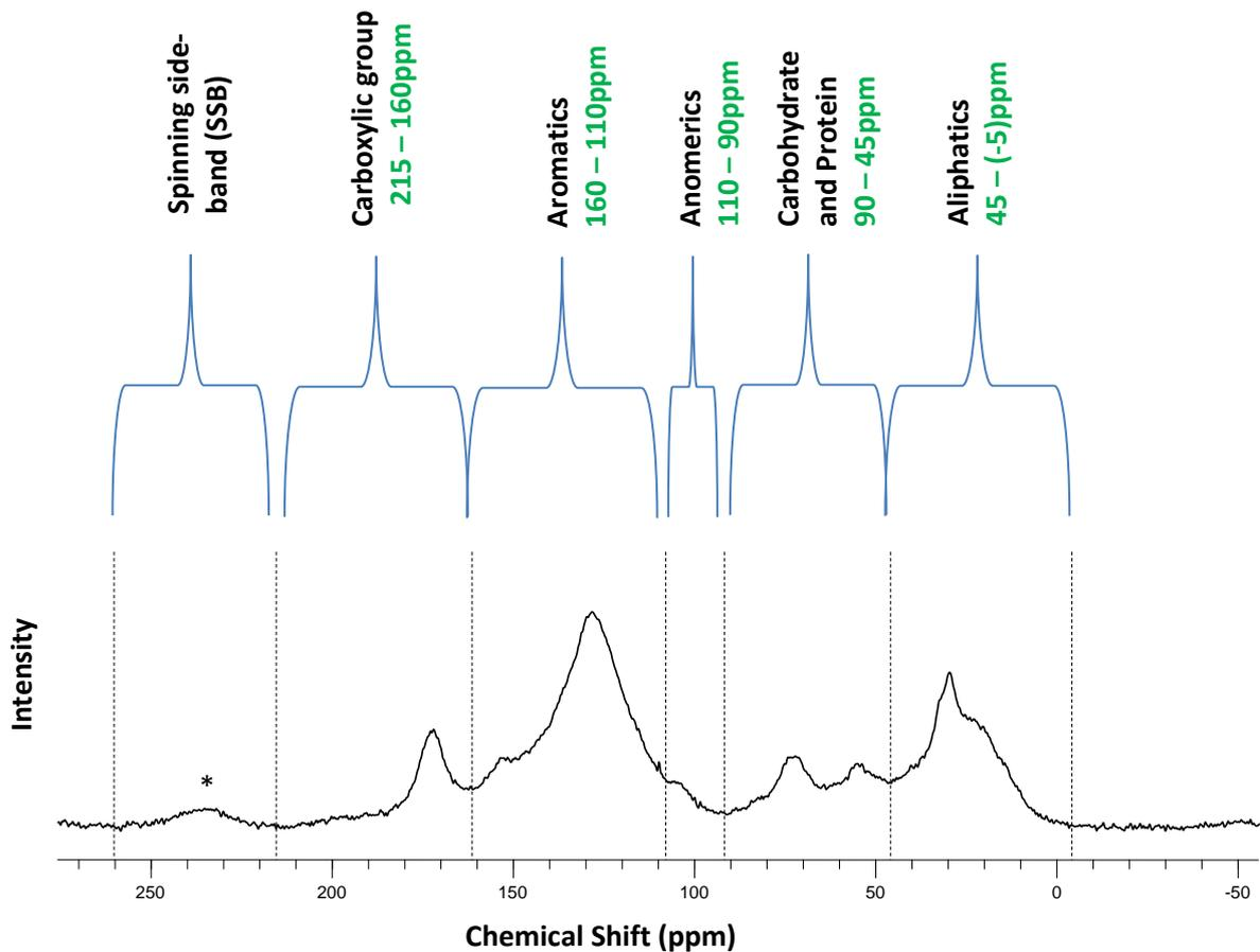
Fig. 3.11. A simplified representation of a typical NMR spectrum of SOM showing various chemical shift regions
