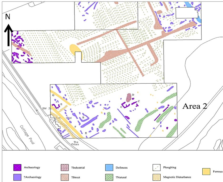
Fig. 7.1. Shows below ground features across the site as identified by GSB prospection ltd (map from GSB prospection, 2004)
