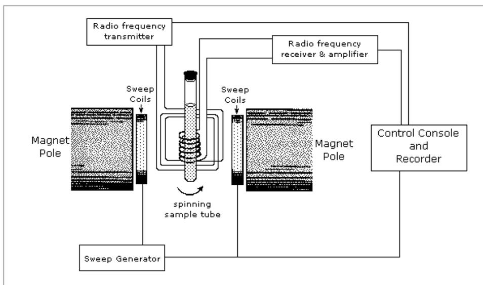
Fig. 3.10. A simplified diagram of the layout of an NMR spectrometer
