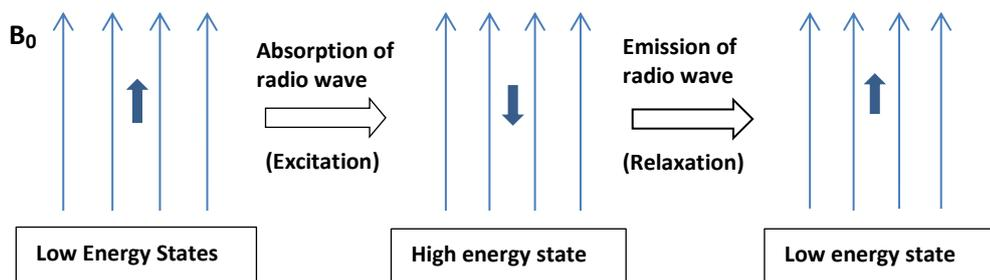
Fig. 3.9. Shows the changes in the state of nucleus (excitation and relaxation) on exposure to radio waves ( $B_0$  – thin blue lines indicate direction of external magnetic field)
