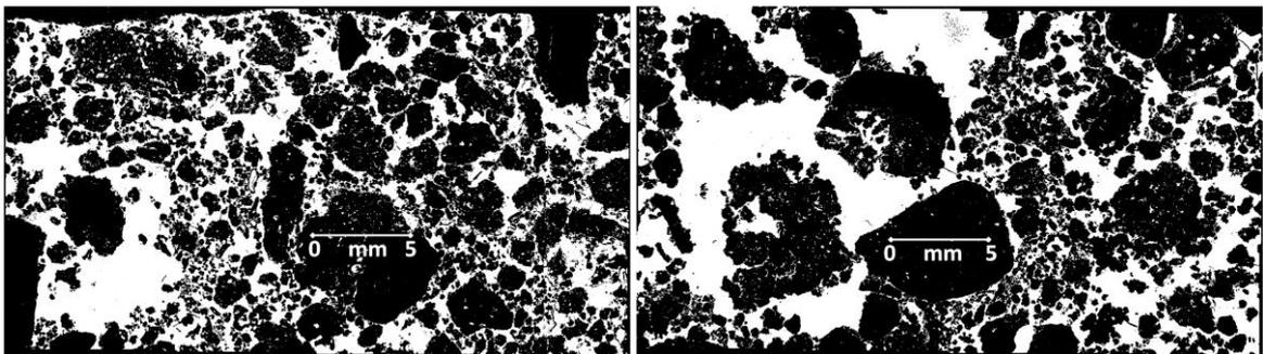
Stump hole sample (upper), depth ~1-10 cm, pore space = 36.0%.
