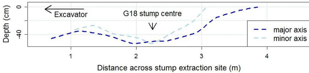
**Figure 6-25: Surveyed profile of non-raked stump.** The indicated direction of the excavator is relative to the major axis only, with the minor axis being orthogonal to this.
