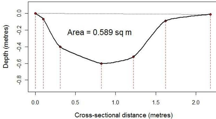
**Figure 4-38: Cross section of spoil trench located within Trench Mounded zone.**
