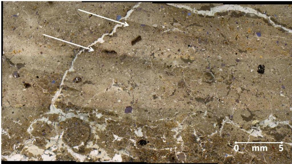
**Figure 5-39: Composite cross-polarised and natural light image of compressed soil.**
