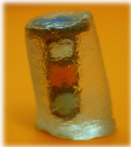
**Figure 6-3: SMTD prior to pre-placement in ground. Height: 25 mm, Diameter: 18 mm.**
