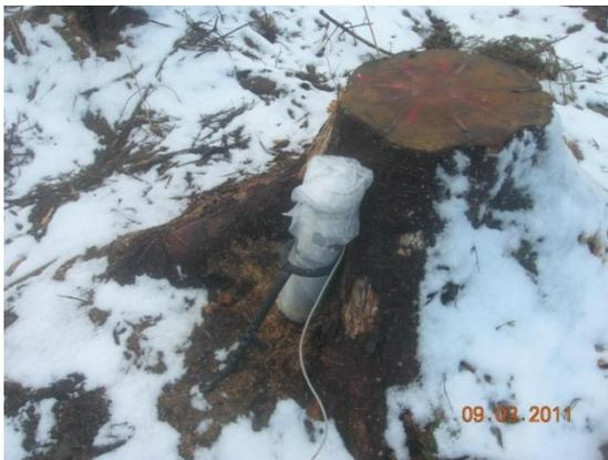
**Figure 4-39: Example of a BS transect point from the Harvested survey with the NaI detector in place.**
