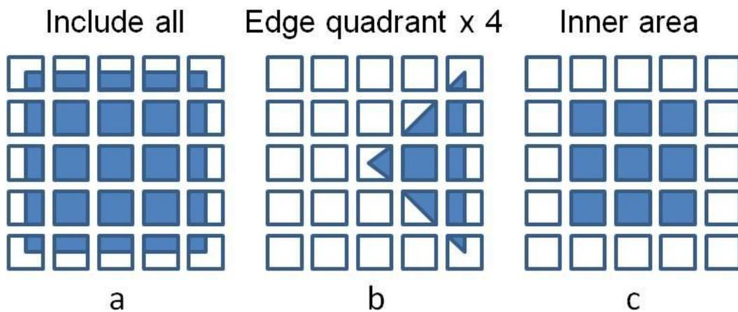
**Figure 6-28: Patterns of placement point inclusion for the calculation of the volume of stump extraction material.** Each bounded square represents an area of 0.75 x 0.75 m centred on each point in the placement array.
