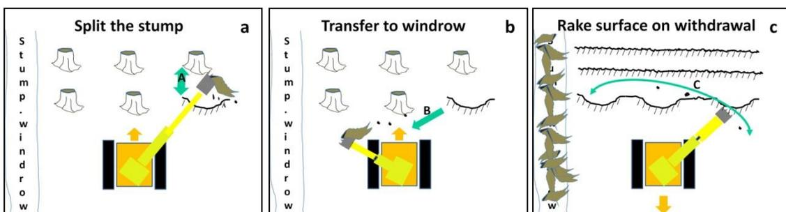
**Figure 6-2: Destumping operational processes.**
