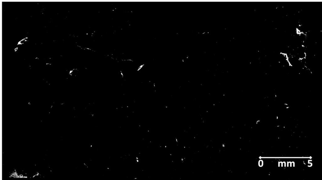
**Figure 5-26: Binary image from DS2, disturbed organic soil at 20 cm depth, pore space 0.4%.**
