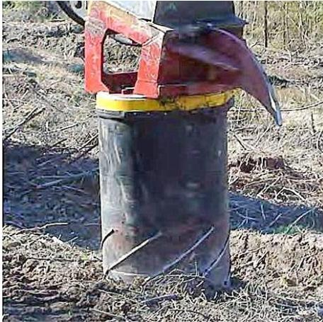
**Figure 7-2: Rotary stump corer.**
