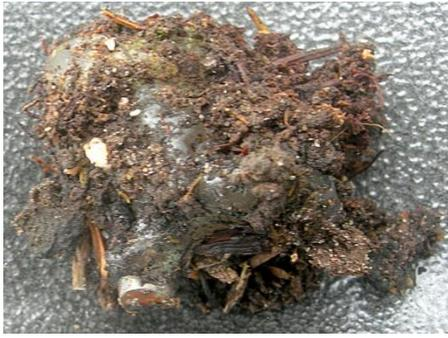
**Figure 6-5: Recovered SMTD, showing gel coating infiltrating adjacent soil.**
