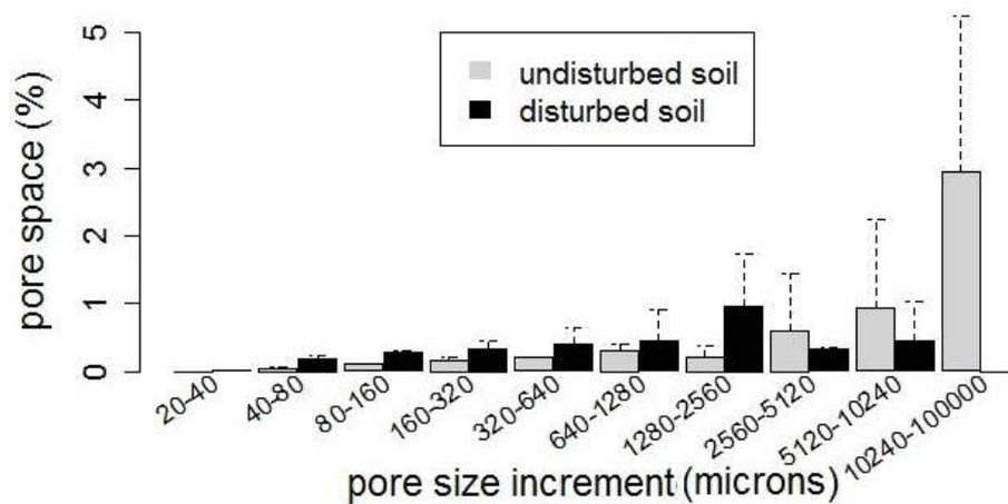
**Figure 5-31: Comparison of pore space between adjacent compressed and non-compressed samples by pore size increments.** Pore size measured by “max Feret” factor, this being the distance between the two most distant points of a connected void, at any orientation. For linear pores this will measure pore length rather than pore width. Dashed lines indicate the standard deviations for pores in each size range.
