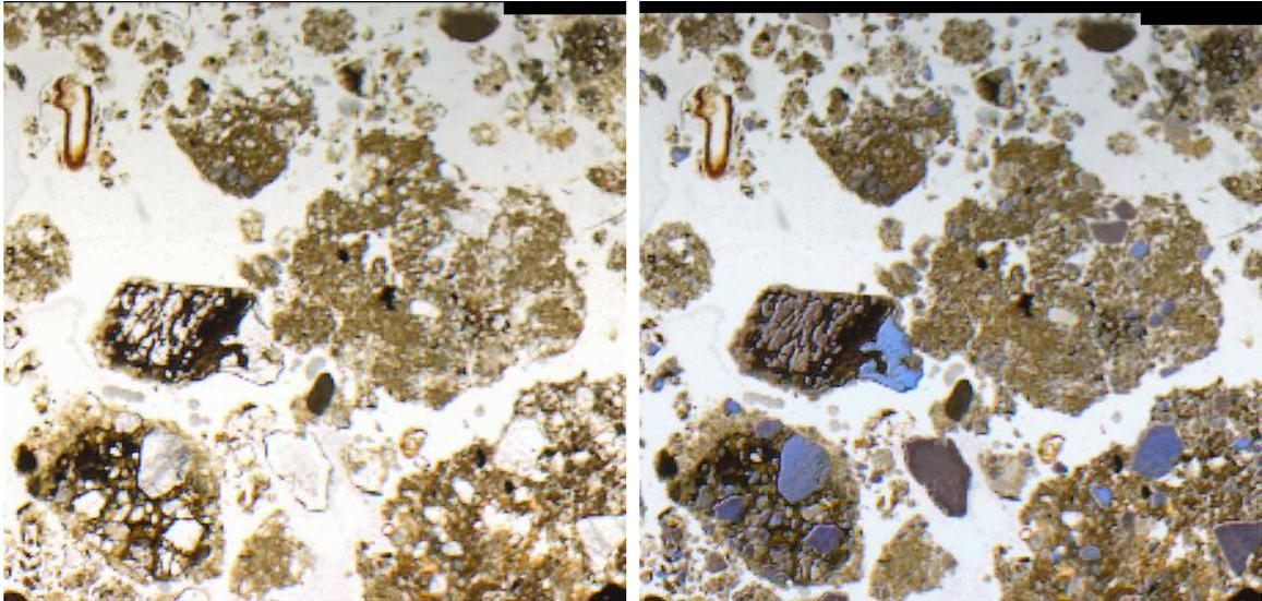
**Figure 5-7: Natural light image (left) and composite image (right) illustrating the effect of the cross polarisation process in distinguishing transparent minerals from void space.**
