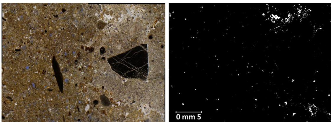
Figure 5-24: Combined polarised and natural light image (left) and binary image from trench DS3, undisturbed soil at 47 cm depth, pore space 0.6%.
