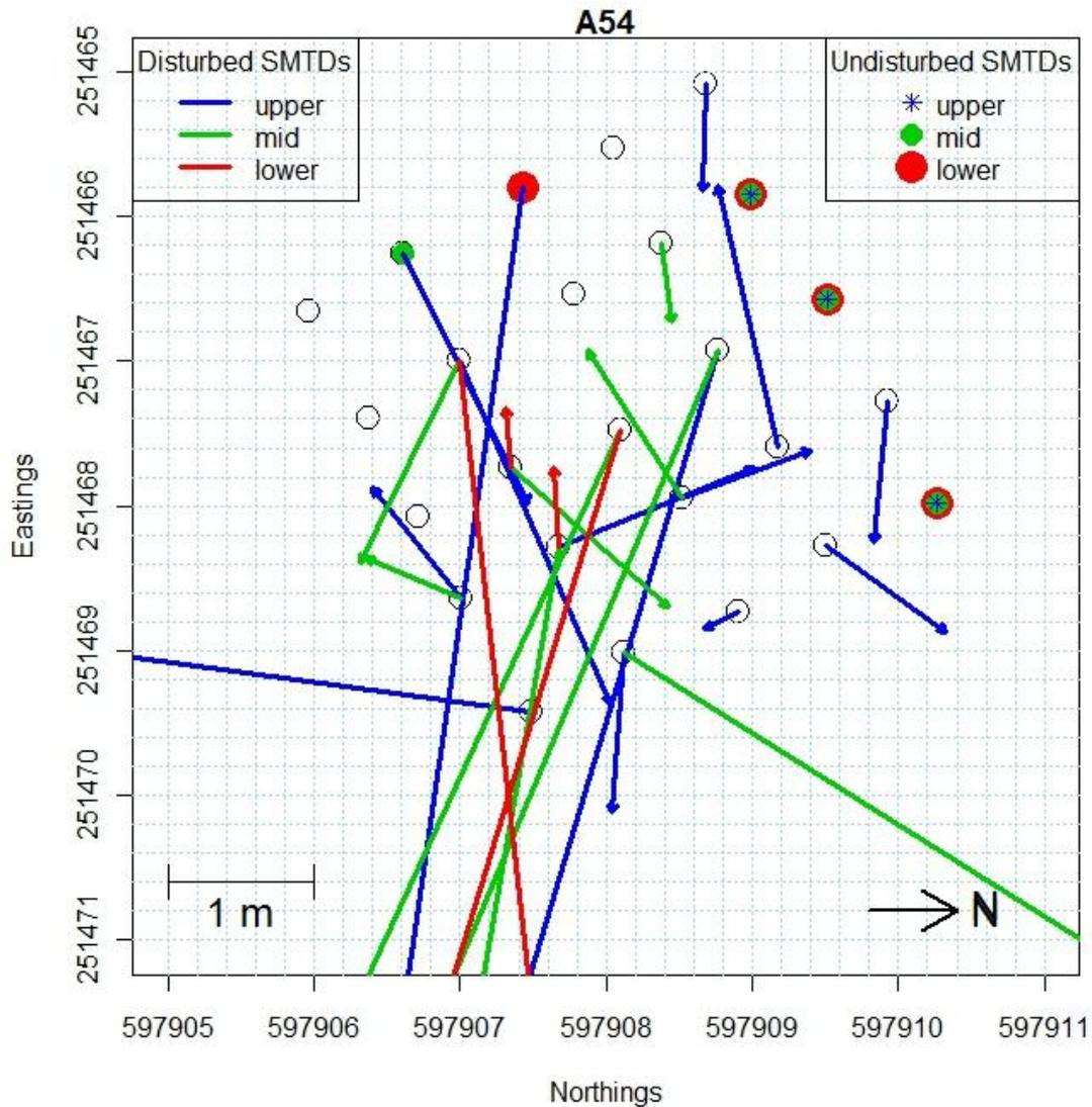
**Figure 6-14: SMTD recovery diagram for stump site A54.** Open circles indicate initial placement positions. Arrows indicate movement path of disturbed SMTDs, coloured by initial burial depth. Circular markers indicate undisturbed SMTD recovery at initial placement site.
