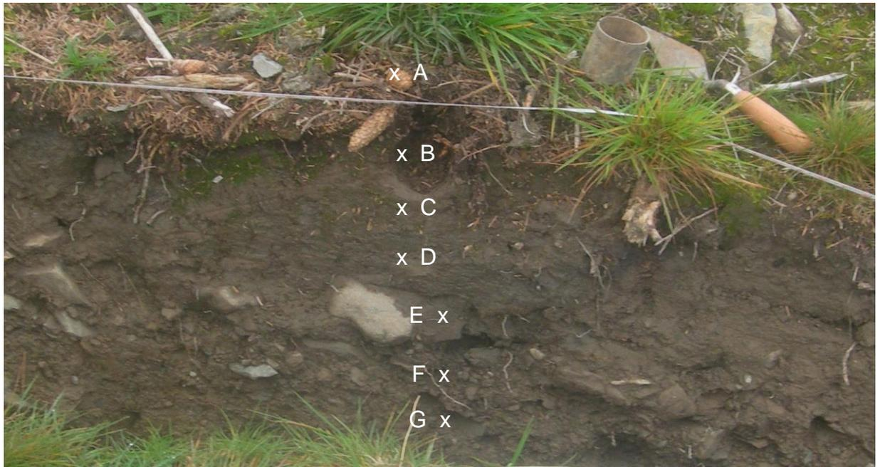
**Figure 5-4: Soil trench DP1 with approximate position of bulk density sample sites indicated.**
