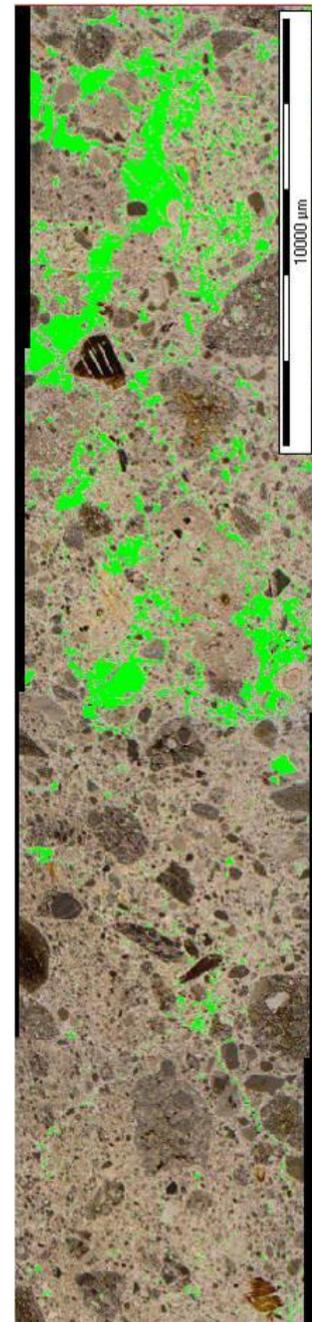
**Figure 5-10: Vertical image from thin section slide TM3A/B. Void space indicated in green.**
