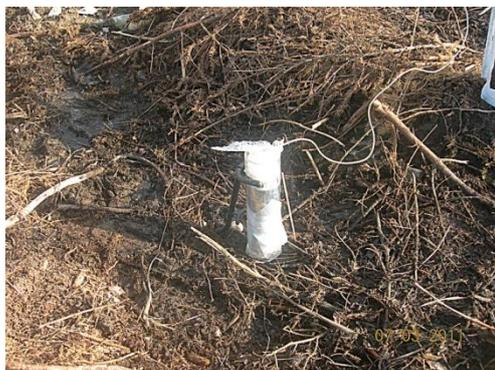
**Figure 4-32: NaI detector in extraction rack.**
