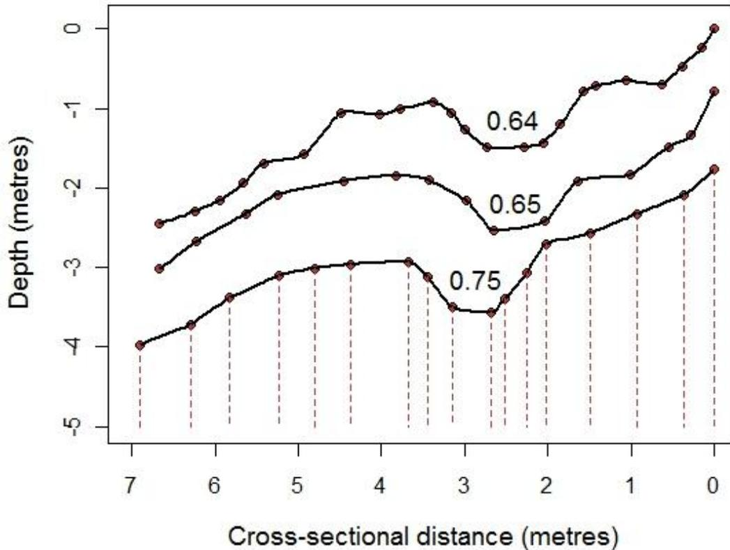
**Figure 5-37: Profile of drain excavations at three points.** Drain spoil was deposited down slope of the profile. Average depth of the drain from adjacent shoulders of each profile is indicated in metres. Profile depths are all relative to the top of the upper profile, with the profile separation indicative of the slope of the drain bed. Profiles were surveyed approximately 40 metres apart.
