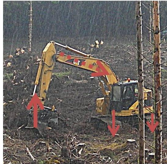
Figure 5-2: Schematic of stump extraction forces.
