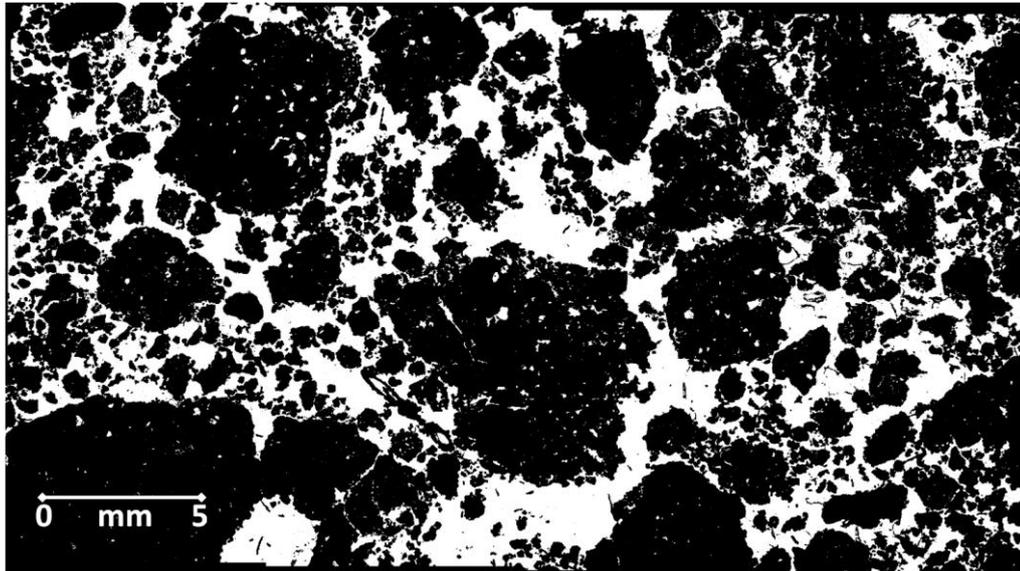
Figure 5-23: Binary image from Stump hole site, depth 1-5 cm, pore space 36.9%.
