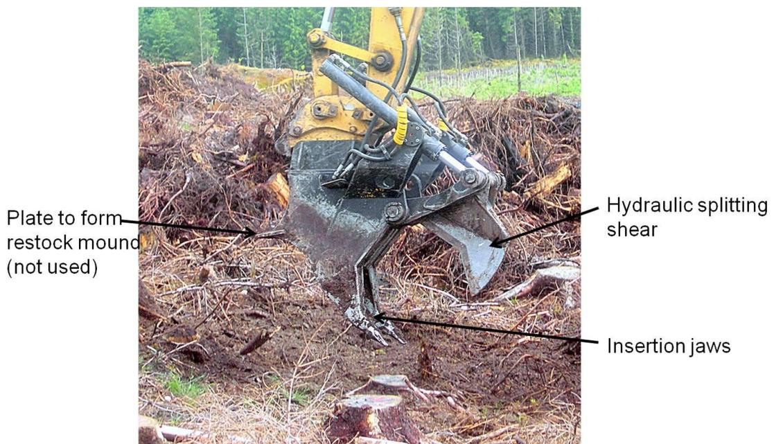
Figure 2-20: Destumping shear head.
