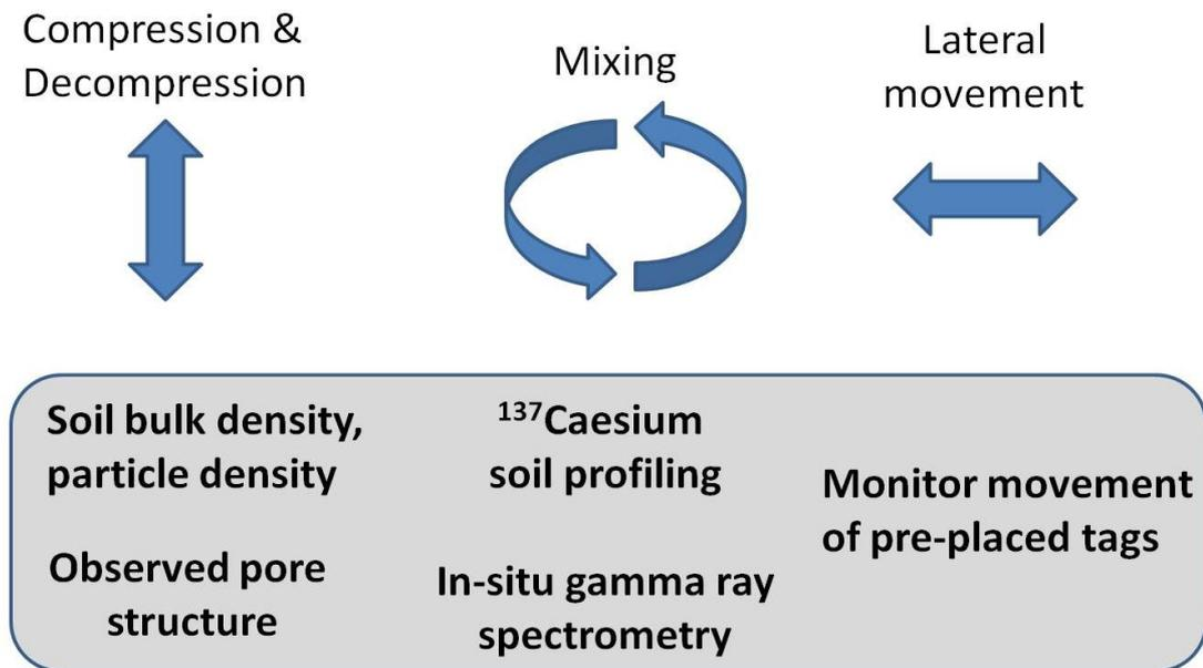
Figure 1-1: Forces causing disturbance.
