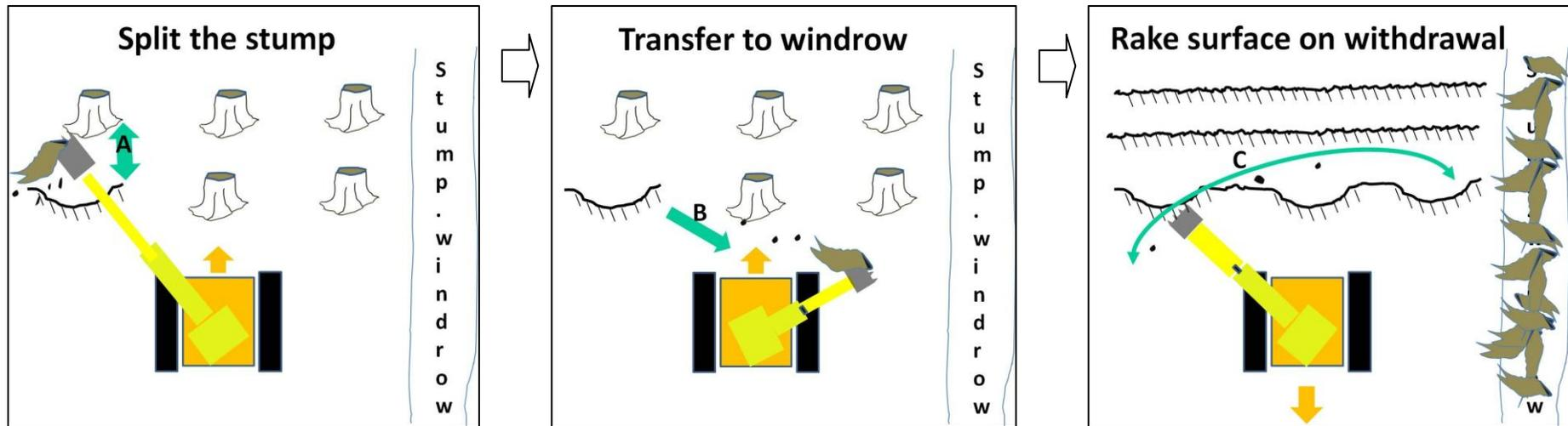
**Figure 2-30: Excavator operational sequence when destumping, based on observations at Lamloch forest.** The stump is initially lifted and split. Stump fragments are transferred to the stump windrow. On withdrawal, the surface is raked over.
