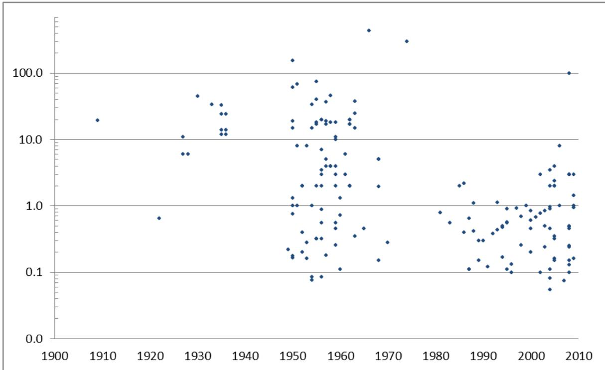
**Figure 5.0: Historical hydropower development in Scotland, scheme capacity (MW) and year of construction (excluding micro schemes)**
