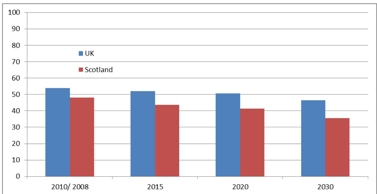
**Figure 3.26: Generation grid system capacity factor (%) for Scotland and the UK, under corresponding moderate renewables uptake scenarios up till 2030**
