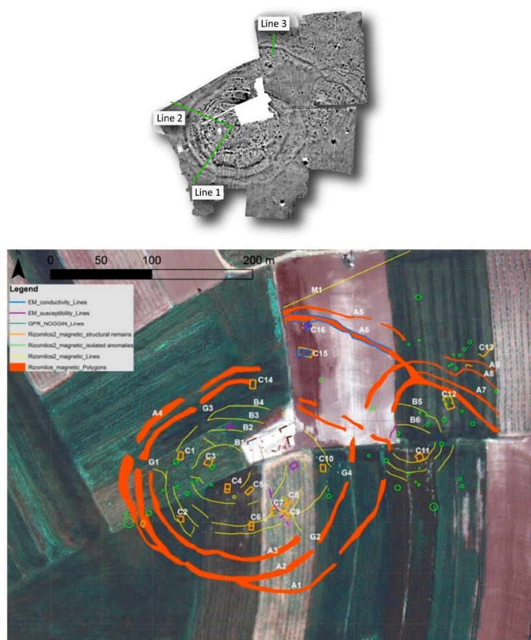
Figure 6. Annotation of the anomalies of interest detected by the geophysical survey at Rizomilos (modified from [19]). The inset at the top shows the related magnetometer results. The grayscale range is the same as that plotted in Figures 1 and 2.
