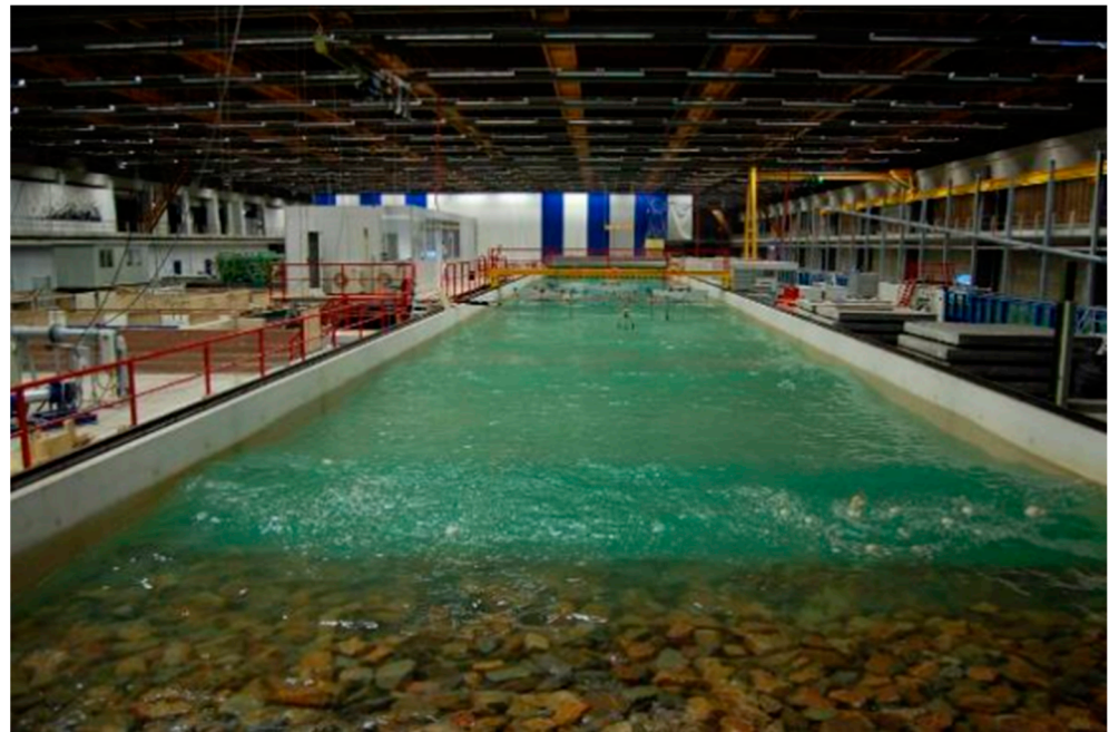
Figure 1. Atlantic Basin (i.e., Deltares' wide wave-current flume), looking from the wave spending beach towards the test section in the middle of the basin and the wave paddles at the end of the basin.
