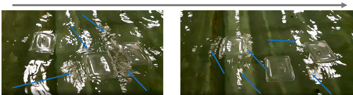
Figure 9. Still images from camera footage of the plastic lids moving on the water surface. The blue arrows highlight capillary wave generation from the objects interacting with the waves. The grey at the top of the figure indicates the direction of wave movement.
