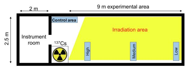
Fig. 1. Schematic diagram of the radiation facility with a <sup>137</sup>Cs source. Shelving units (blue boxes) were placed in the path of the radiation source, as well as in a zone outside the radiation area (control area).
