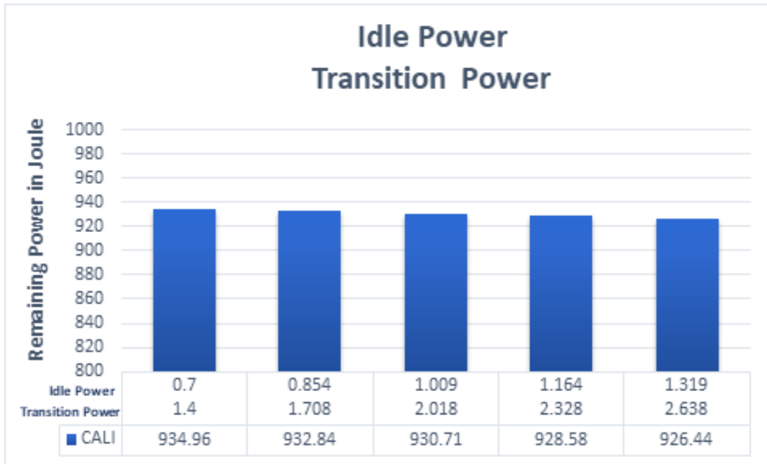
Figure 7. 13: Levels of energy consumption of CALI in buffering mode against the value variations of idlePower and transitionPower energy parameters
