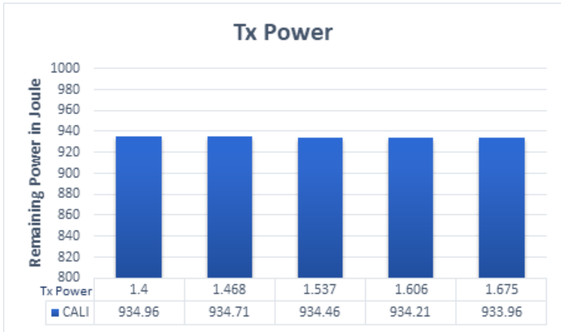
Figure 7. 11: Levels of energy consumption of CALI in buffering mode against the value variations of txPower energy parameter
