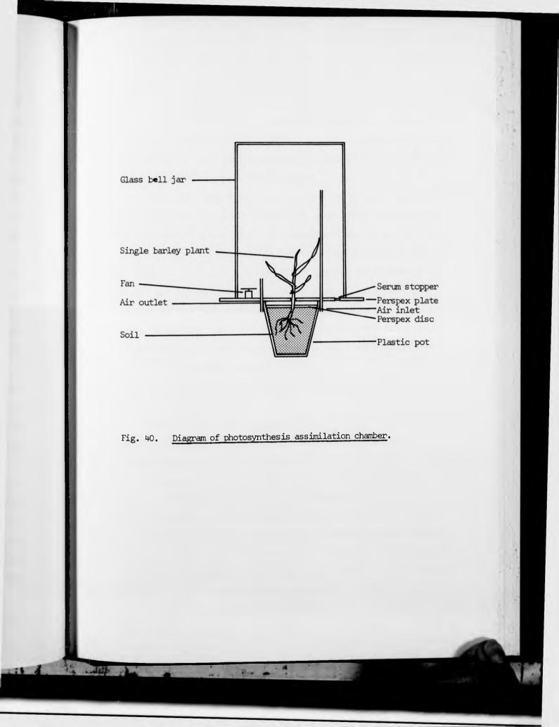
obtained. The assimilation chamber was sealed off from the rest of the circuit and the plant exposed to  $^{14}CO_2$  for 30 minutes as described in the following section. After this presentation period, the chamber was reconnected to the IRGA and a second photosynthesis reading obtained as above. The values of net photosynthesis presented (in mg C h<sup>-1</sup>plant<sup>-1</sup>) are the means of these two readings.
