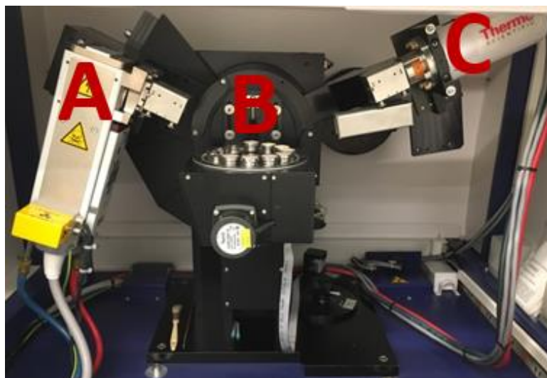
Figure 2.30 - X-ray diffractometer with X-ray tube (A), sample holder (B) and X-ray detector (C)
