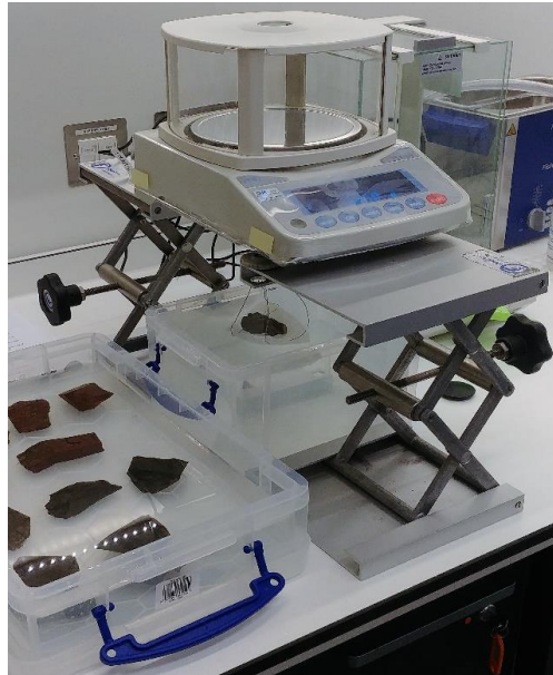
Figure 2.15 - Sample being weighed under water by hanging a cradle from the underside of the weighing scales and placing the specimen in the cradle submerged under water
