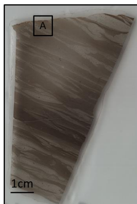
Figure 5.55 - Scan of BC3 (11) showing the locations of SEM-EDX mapping, focussing a potential dissolution area at the surface
