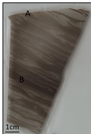
Figure 5.30 - Petrographic thin section scan of BC3 (11), with A focussing on the sample surface and B focussing on a vertical microcrack at depth
