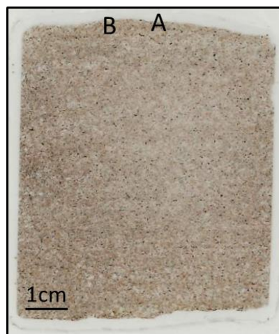
Figure 4.23 - Petrographic thin section scan of CB3 (9), with A and B focussing on two areas of the sample surface
