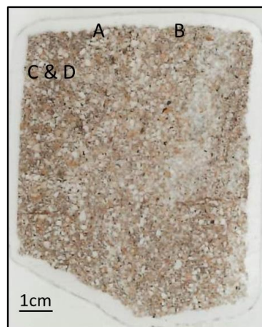
Figure 4.19 – Petrographic thin section scan of CB1 (1), with sites A and B focussing on fractured quartz grains while C and D focus on a lateral microcrack
