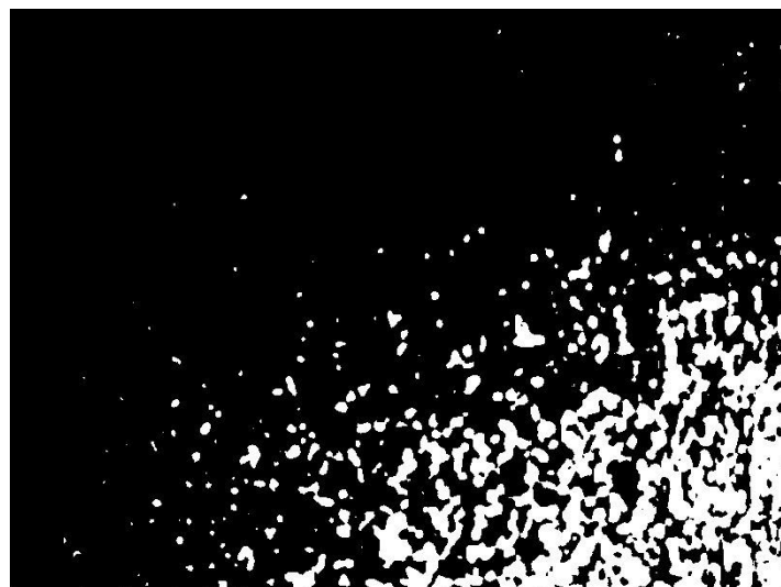
Figure 4.122 - BB2 (5) mapped section (A) auto-threshold image of Mg distribution. The map has been rotated and cropped to the immediate surface of the sample
