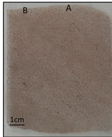
Figure 5.14 - Petrographic thin section scan of CB2 (7), with A and B focussing on two areas of the sample surface
