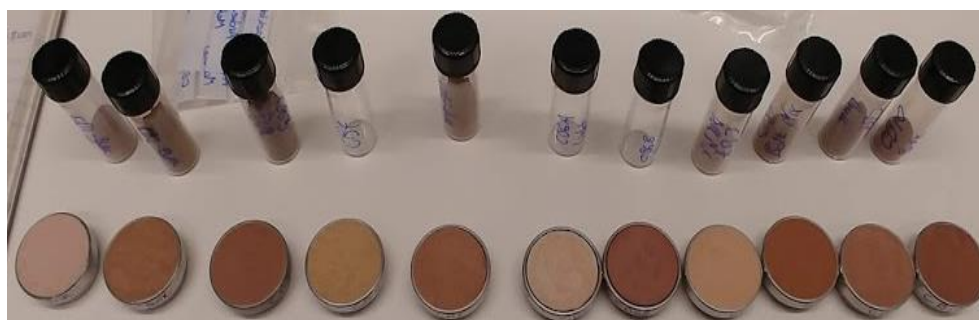
Figure 2.31 - Fine powder Torridonian Sandstone samples in their sample holders before XRD analysis
