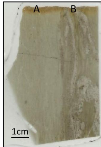
Figure 4.42 - Petrographic thin section scan of BC3 (8), with A and B focussing on two areas of the sample surface where dolomite dissolution appears prevalent
