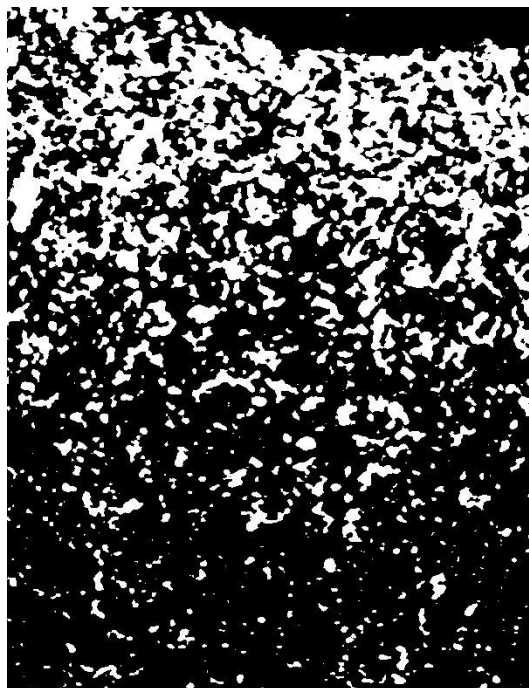
Figure 4.120 - BC3 (8) mapped section auto-threshold image of Fe distribution. The map has been rotated and cropped to the immediate surface of the sample
