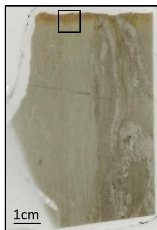
Figure 4.89 - Scan of BC3 (8) showing the location of SEM-EDX mapping, focussing on the surface exposed in the CEF
