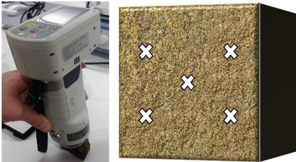
Figure 2.28 - Konica Minolta Chroma Meter CR-400 being used to determine sample surface colour. Sample locations marked on exemplar block
