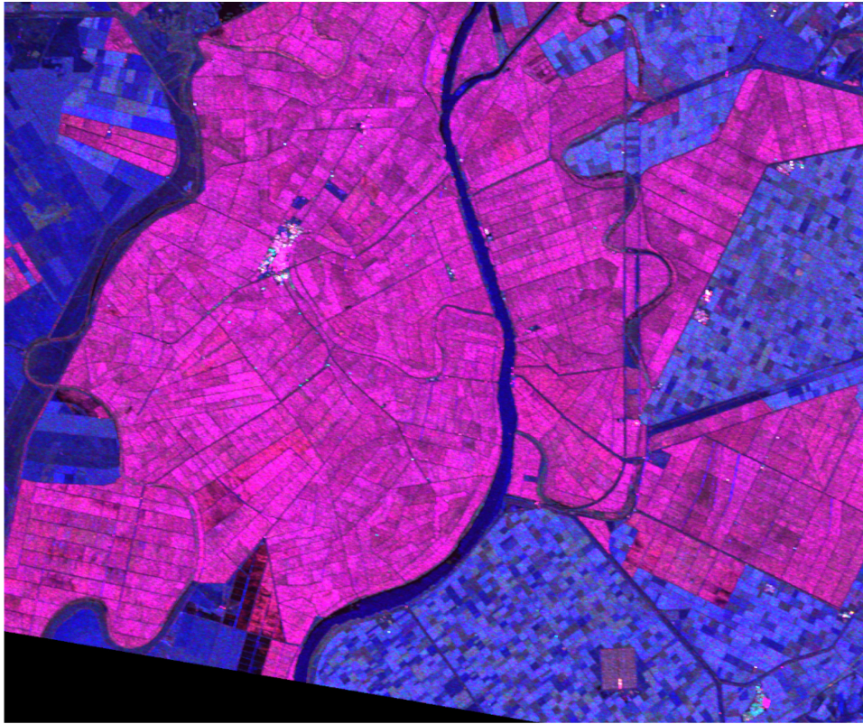
Fig. 1. Rice fields in the south of Spain (Test site 1). Quad-Pol RADARSAT-2 image acquired the 02/08/2014. Blue: \sqrt{\lambda} \cos(\alpha) , Red: \sqrt{\lambda} \cos(\alpha) \sin(\beta) , Green: \sqrt{\lambda} \sin(\alpha) \sin(\beta) . See (9).
