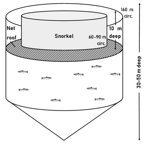
Figure 1.5. Schematic of a commercial snorkel cage (modified from Wright et al., 2017).
