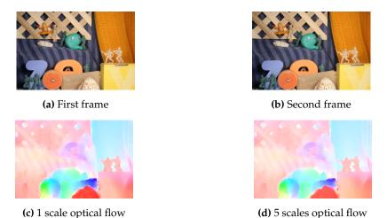
**Figure 12.** Optical Flow results using the implementation from [40]. (a,b): source frames. (c): output from 1 scale optical flow (used in our FPGA implementation). (d): output from 5 scales optical flow.
