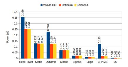
Figure 16. MeanShift Tracking power consumption on Zedboard.
