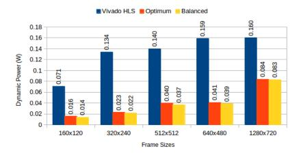
**Figure 9.** Total dynamic power consumption for  $3 \times 3$  sliding window read: Vivado HLS versus proposed methods.
