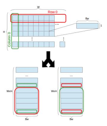
**Figure 1.** Mapping a 3-D array into row-major and colum-major order 2-D arrays.
