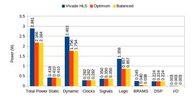
**Figure 13.** TV-L1 Optical Flow power consumption on Virtex 7.
