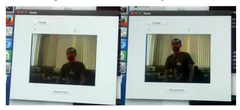
**Figure 15.** MeanShift Tracking: real-time face tracking displayed on PC. Image sent from Zedboard over Ethernet connection.
