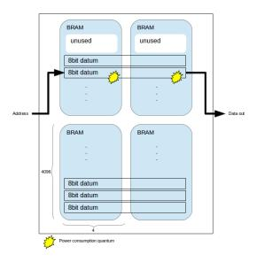
Figure 3. Partitioning across two BRAMs horizontally. Each access consumes two power consumption quantums.
