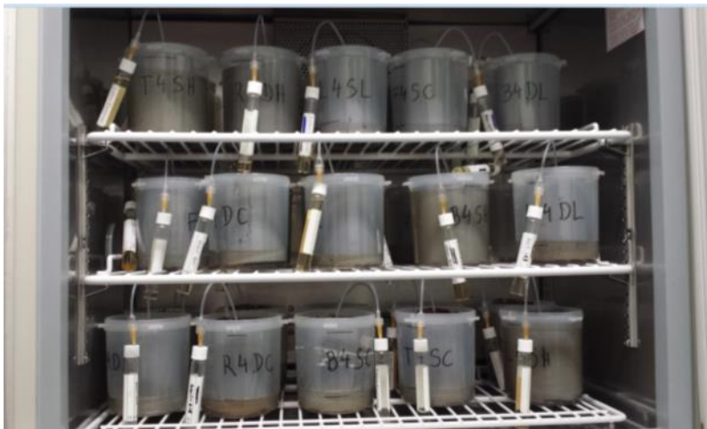
Figure 4.1 Peat cores in their plastic tubs in the incubator. Rhizon samplers are inserted here with evacuated glass vials attached.
