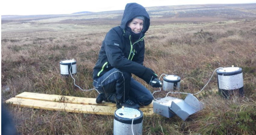
Figure 2.4 Gas sampling for GHG flux calculations in action; chambers are visible, with tubing towards sampler who in this way is able to stay on the platform to avoid disturbance.
