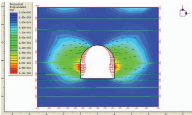
**Figure 5. Maximum tunnel wall displacement.**
