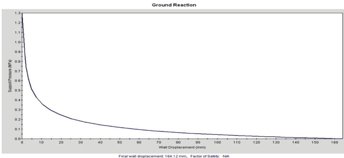
Figure 2. Ground reaction curve drawn using the Duncan-Fama method.
